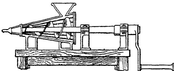
FIG. 37. —Cartridge Mixing Machine for Gelatine Explosives.
