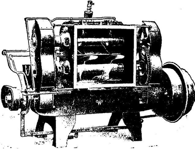
FIG. 35. — Messrs Werner, Pfleiderer, & Perkin's Mixing Machine.
