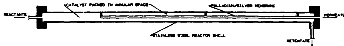
Figure 1 Scale drawing of the original TSTA proof-of-principle PMR
