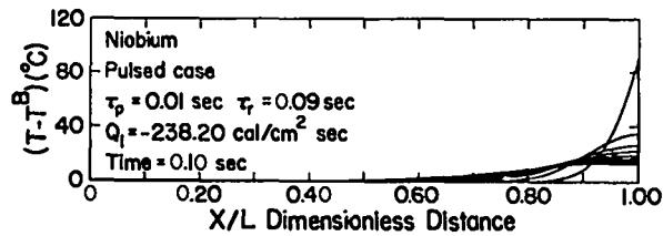
Fig. 5. Temperature profiles in a 1 cm thick Niobium wall with an incident flux of 238.2 cal/cm<sup>2</sup> sec (1 kW/cm<sup>2</sup>). Each line represents .01 sec of elapsed time.
