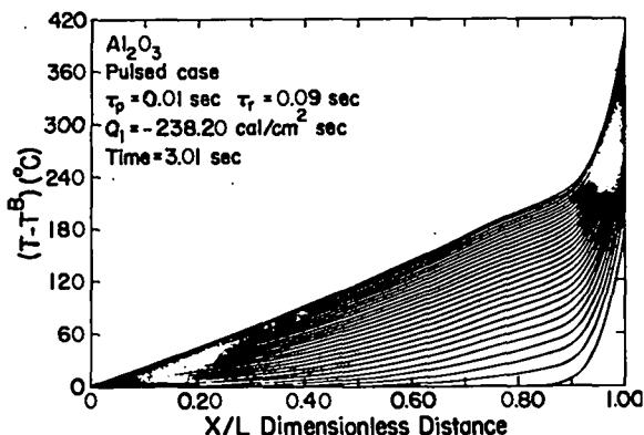
Fig. 7. Temperature profiles for a .5 cm  $\text{Al}_2\text{O}_3$  wall with an incident flux of  $238.2 \text{ cal}/\text{cm}^2 \text{ sec}$  ( $1 \text{ kW}/\text{cm}^2$ ). Approach to a steady state temperature distribution after 31 pulses with each line appearing at the end of every pulse. ( $\Delta t = .1 \text{ sec}$ ).
