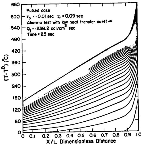
Fig. 11. Temperature profiles for a 1 cm  $\text{Al}_2\text{O}_3$  wall with an incident wall flux of 238.2 cal/cm<sup>2</sup> sec (1 kW/cm<sup>2</sup>) and a low liquid Li heat transfer coefficient  $h = .14$  cal/cm<sup>2</sup> sec °C. Each line appears at the end of every pulse ( $\Delta t = .1$  sec).
