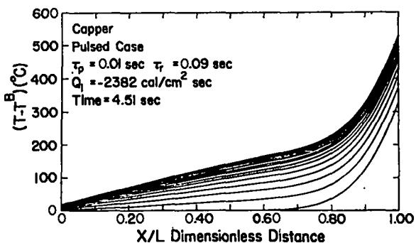
Fig. 4. Temperature profiles in a 1 cm thick Copper wall with an incident flux of 2382 cal/cm<sup>2</sup> sec (10 kW/cm<sup>2</sup>). Approach to steady state temperature distribution after 46 pulses with each line appearing at the end of every pulse. ( $\Delta t = .10$  sec)
