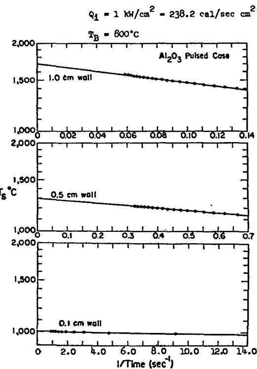
Fig. 8. Surface temperature (inside) of the first wall. Extrapolations to infinite time are shown for a 1 cm, .5 cm, and .1 cm  $\text{Al}_2\text{O}_3$  wall with a loading of  $283.2 \text{ cal}/\text{cm}^2 \text{ sec}$  ( $1 \text{ kW}/\text{cm}^2$ ).
