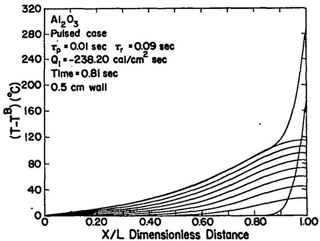
Fig. 9. Temperature profiles for a .5 cm  $\text{Al}_2\text{O}_3$  wall with an incident flux of  $238.2 \text{ cal}/\text{cm}^2 \text{ sec}$  ( $1 \text{ kW}/\text{cm}^2$ ).
