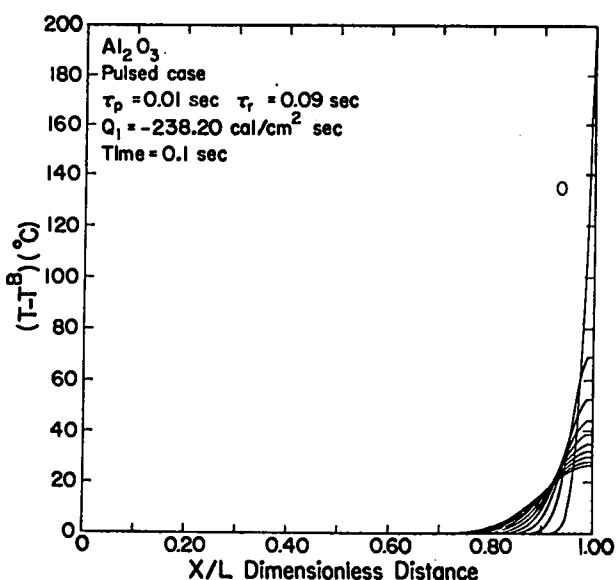
Fig. 1. Temperature profiles in a 1 cm thick  $\text{Al}_2\text{O}_3$  wall with an incident flux of  $238.2 \text{ cal/cm}^2\text{-sec} \sim (1 \text{ kW/cm}^2)$ . Each line represents .01 sec of elapsed time. Line 0 is just after the 1st pulse.
