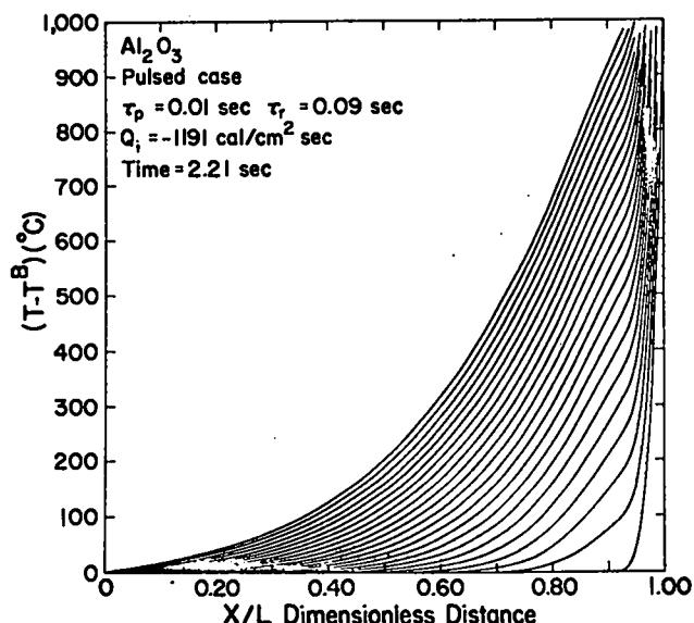
Fig. 2. Temperature profiles in a 1 cm thick  $\text{Al}_2\text{O}_3$  wall with an incident flux of  $1191 \text{ cal/cm}^2\text{ sec} \sim (5 \text{ kW/cm}^2)$ . Each line is drawn at the end of every pulse.
