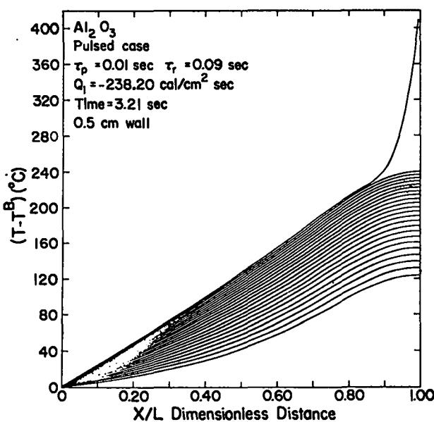
Fig. 10. Temperature profiles for a .5 cm  $\text{Al}_2\text{O}_3$  wall with an incident flux of  $238.2 \text{ cal}/\text{cm}^2 \text{ sec}$  ( $1 \text{ kW}/\text{cm}^2$ ).
