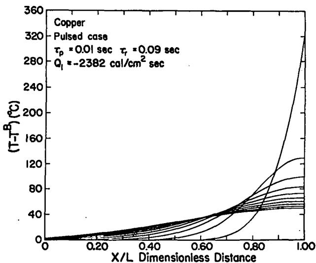
Fig. 3. Temperature profiles in a 1 cm thick Copper wall with an incident flux of 2382 cal/cm<sup>2</sup> sec (10 kW/cm<sup>2</sup>). Each line represents .01 sec of elapsed time.
