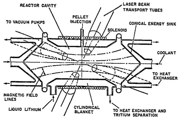
Fig. 2. Magnetically protected wall laser-fusion reactor concept.
