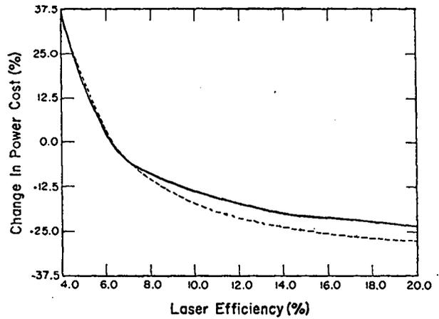
Fig. 5. Effect of laser efficiency on power production cost.
