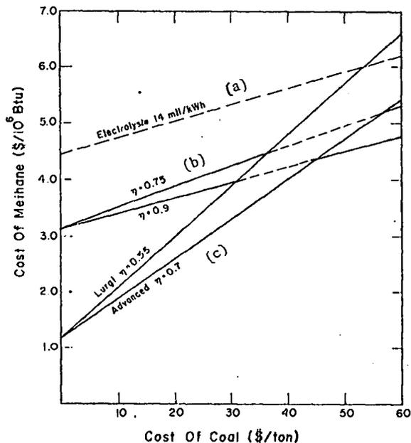
Fig. 11. Costs of producing methane by various methods as functions of the cost of feed coal: (a) electrolytically produced  $H_2$  followed by direct hydrogenation at  $\eta=0.9$ , (b) radiolytically produced  $H_2$  at  $\eta=0.35$  followed by direct hydrogenation with waste heat converted to electricity and sold for 14 mil/kWh, and (c) standard coal gasification ( $\eta$ =efficiency).
