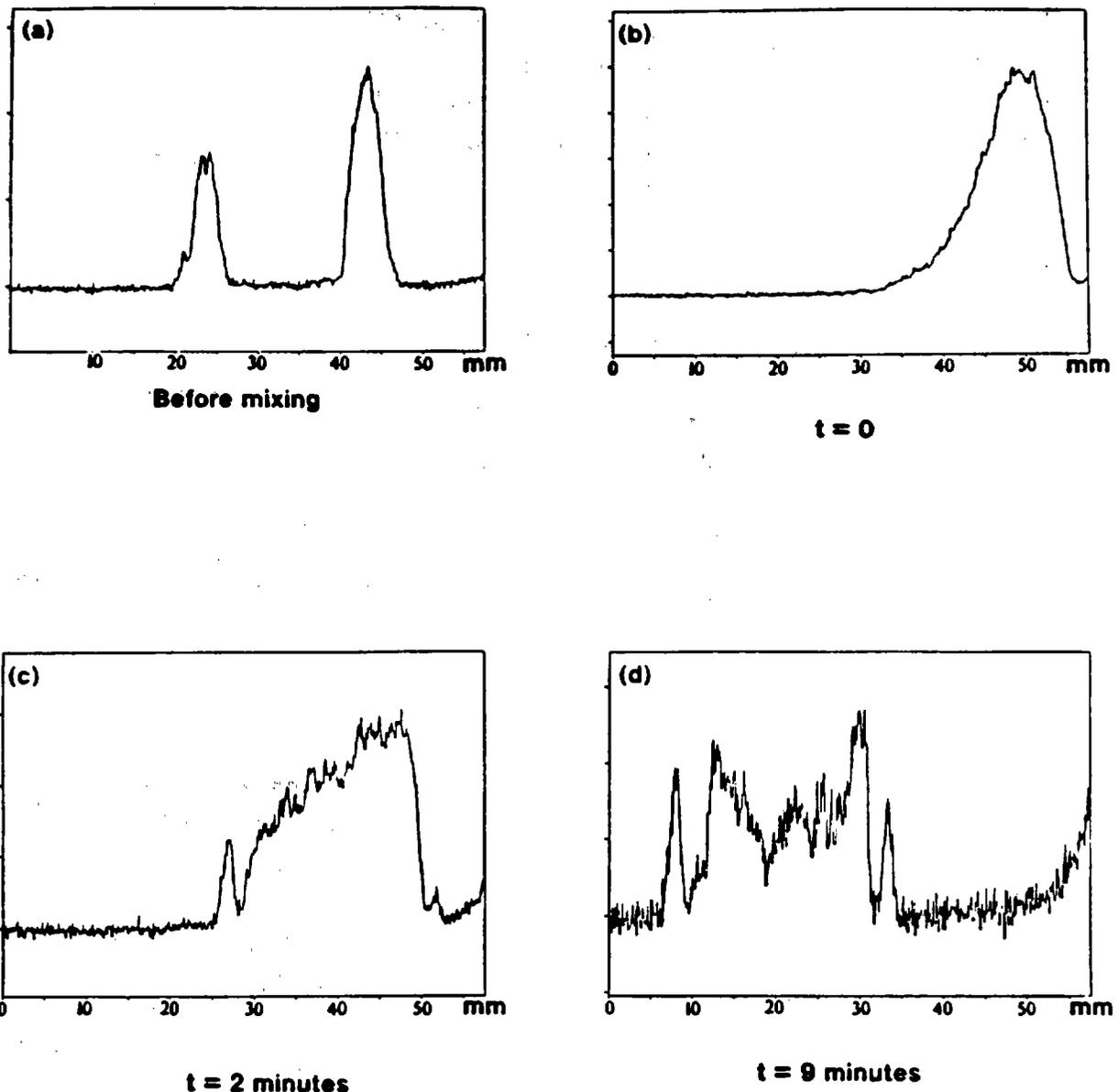
Figure 5. Streak camera data showing back scattering from a 4-ps-wide laser pulse striking a vial of 7- $\mu\text{m}$  copper particles suspended in alcohol. The vertical scales show intensities, but the scales are different for each graph. The horizontal scales show thickness of material traversed. The narrow peaks before and after the main scattering data are from the glass windows. As time after mixing increases, the traces have progressively more of the copper settled out.
