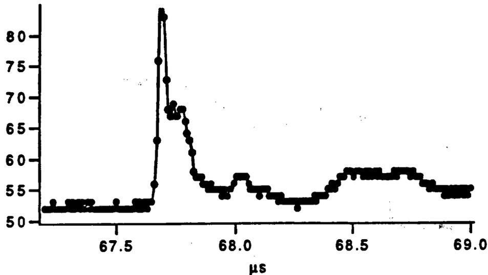
Figure 1. Data from an optical pin in contact with detonating high explosive. The vertical scale is roughly exponential with a peak value of a few hundred microwatts and a noise level of about 0.1  $\mu$ W.
