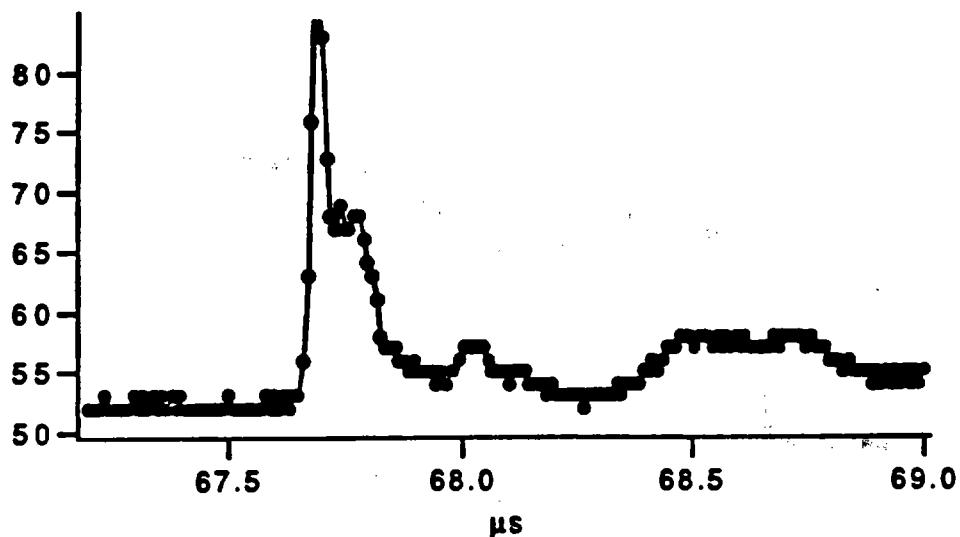
Figure 1. Data from an optical pin in contact with detonating high explosive. The vertical scale is roughly exponential with a peak value of a few hundred microwatts and a noise level of about  $0.1 \mu\text{W}$ .
