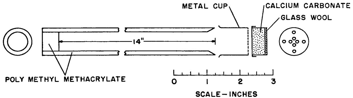
Fig. 2. Special accessories for the steel shell.
