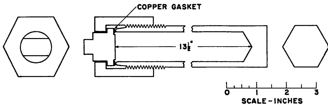
Fig. 1. Steel shell for protection of sealed tube.
