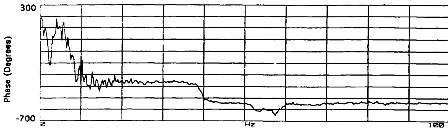
Figure 21. Phase Angle between Driver and Test Unit for the Vibration Technique Qualification Experiment; First Run
