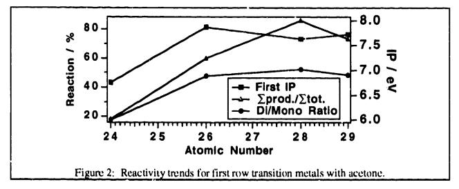
The results of this study show an increase in reactivity ( $\Sigma$ Products /  $\Sigma$ Total) as the ionization potential of the specific metal reagent ion increases, for both mono- and bi-adduct formation. This observation is consistent with the findings of other researchers <sup>9</sup>, who conclude that the 1P of gas phase metal ions is directly related to their observed gas phase reactivity.
