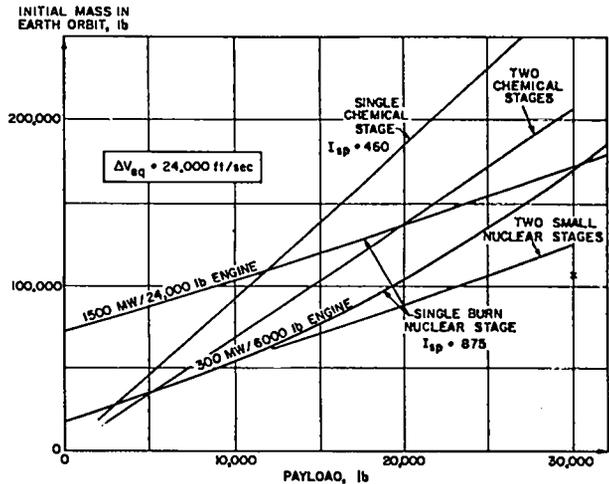
Fig. 6. Vehicle mass requirements for a 24 000 ft/sec mission.
