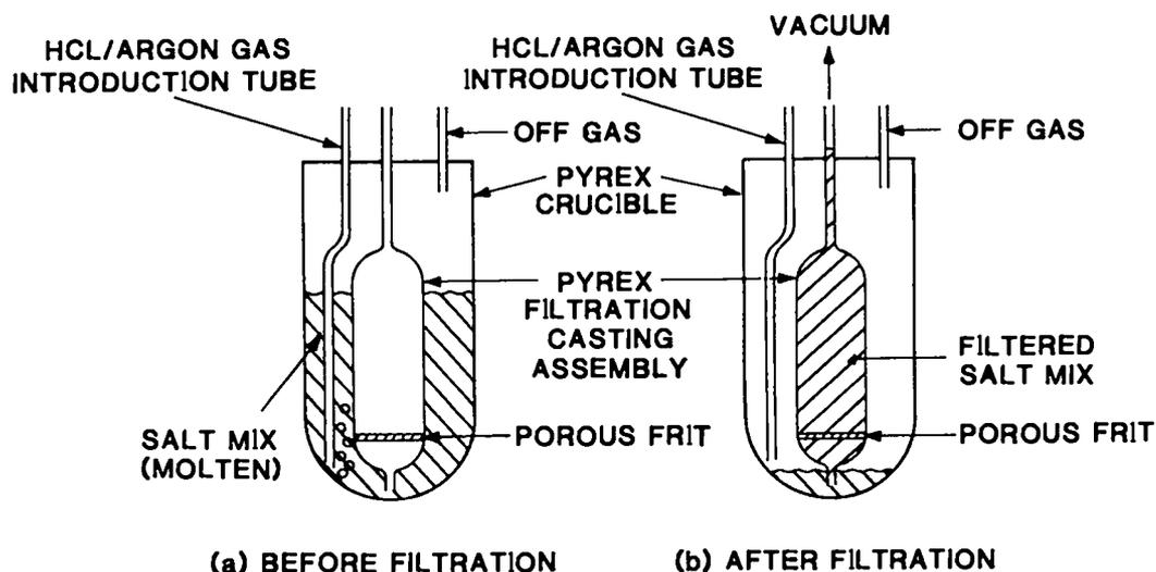
Fig. 2. Batch pyroredox salt production apparatus.
