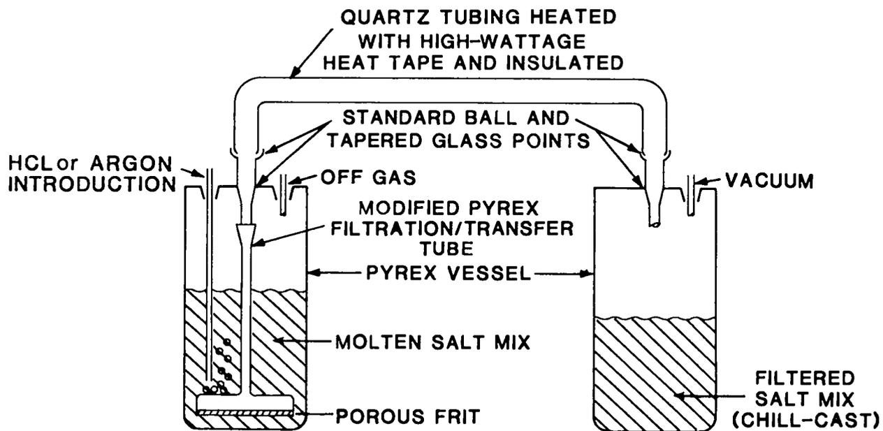
Fig. 8. Apparatus used in semicontinuous pyroreodox salt preparation.
