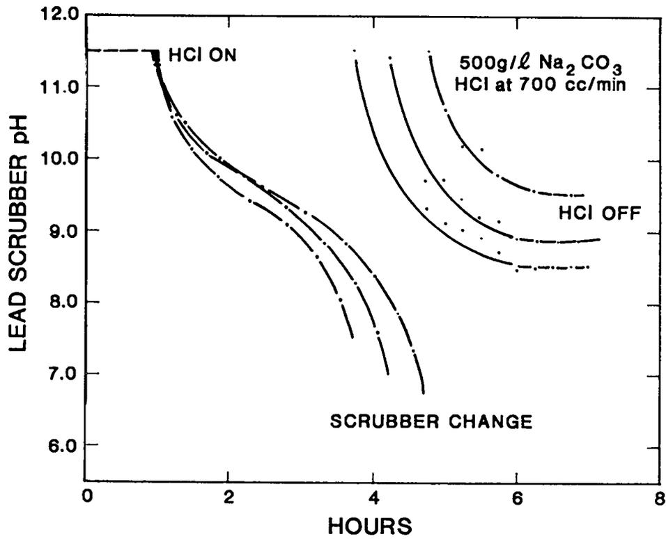
Fig. 6. Neutralization of scrubber solution with anhydrous HCl.
