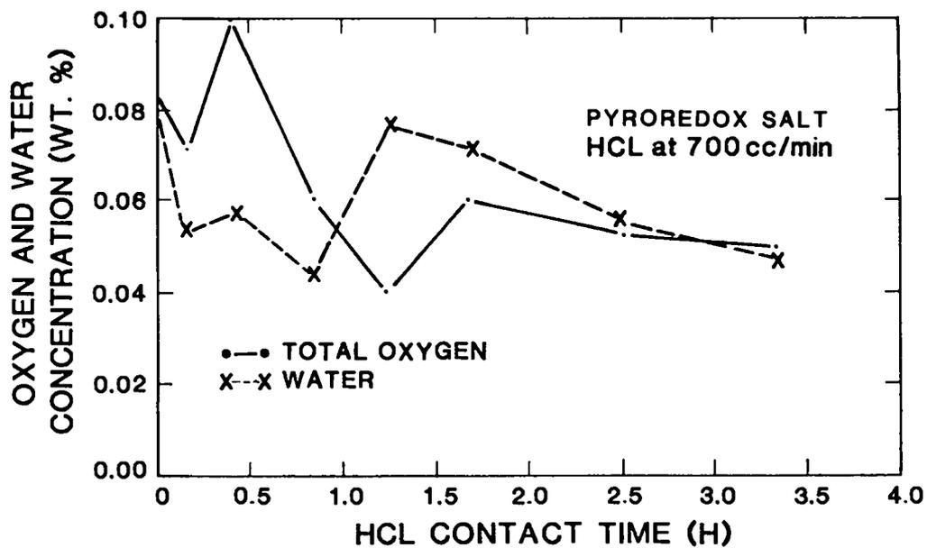
Fig. 4. Total oxygen and water in pyroredox salt as a function of HCl gas contact time.
