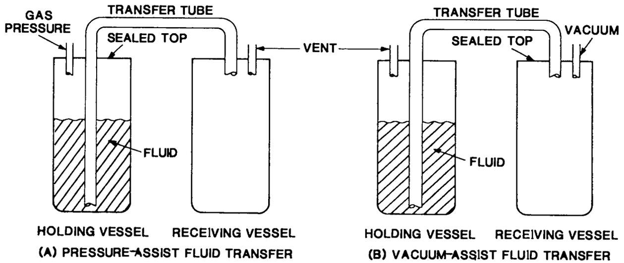
Fig. 7. Schematic of pressure-assist and vacuum-assist fluid transfer.
