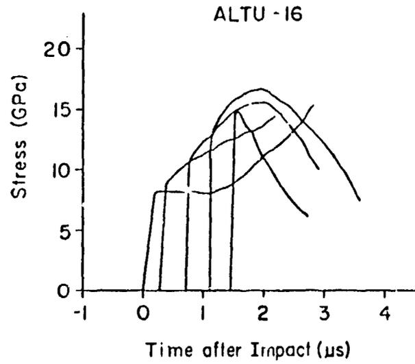
Fig. 8. Manganin gauge records in ALTU-16 propellant. First gauge is on interface between copper flyer and ALTU-16. Subsequent gauges were embedded at 2, 4, 6, and 8 mm. Run to detonation is 10 mm. (From Ref. 4)
