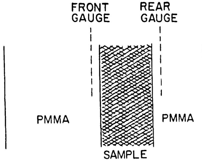
Fig. 3. Schema of the sample and gauge configuration. The manganin gauges are 0.75 mm from the sample. The shock moves from left to right.
