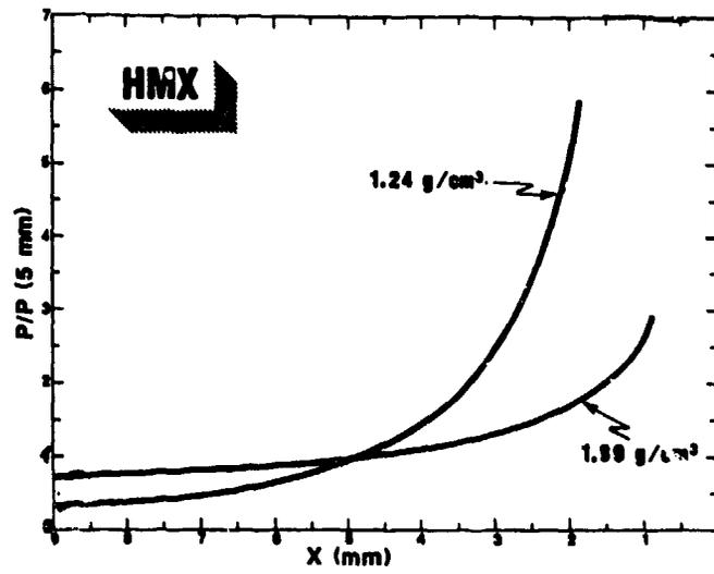
Fig. 6. Common-curve buildup for two densities of HMX.
