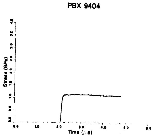
Fig. 7. Transmitted profile for a PBX 9404 sample 6.4 mm thick.
