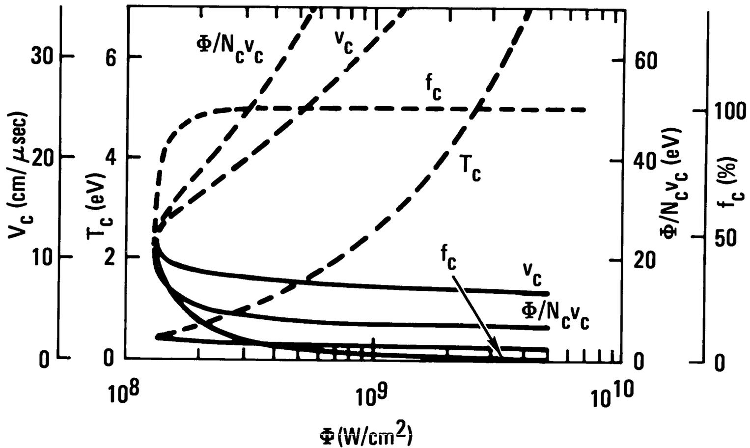
Fig. 1 Hydrogen ablation velocity  $v_c$ , temperature  $T_c$ , and degree of ionization  $f_c$  at critical surface, and energy absorbed per particle ablated  $\Phi/N_c v_c$  versus absorbed laser flux. Solid curves are lower-ionization-branch solutions; dashed are higher-ionization-branch solutions.
