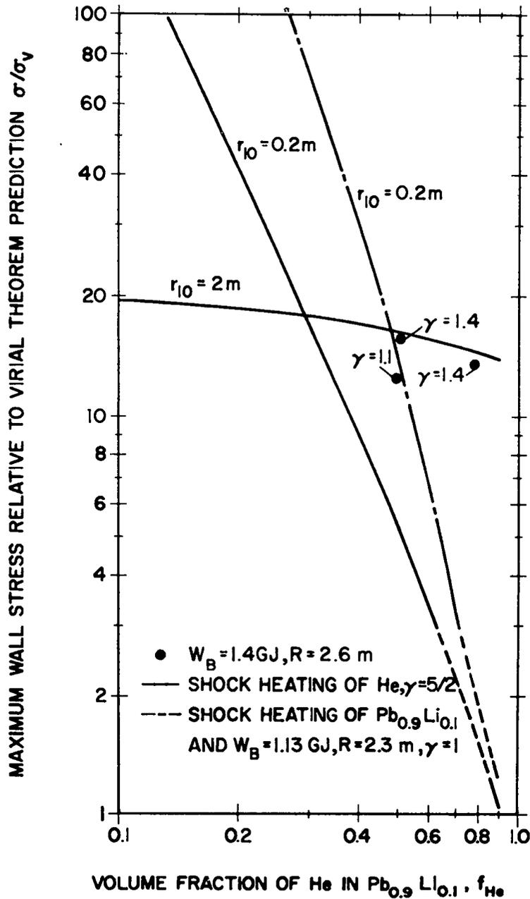
Fig. 4 Dependence of maximum wall stress relative to predictions of the virial theorem as a function of the bubble void fraction. The energy released at the center of the spherical vessel is  $W_B$ , the vessel radius is  $R$  and the specific heat ration of the gas is  $\gamma$ . Shown also as points are results for similar conditions from the hydrodynamic code PAD. (Ref. 10, Sec.V).
