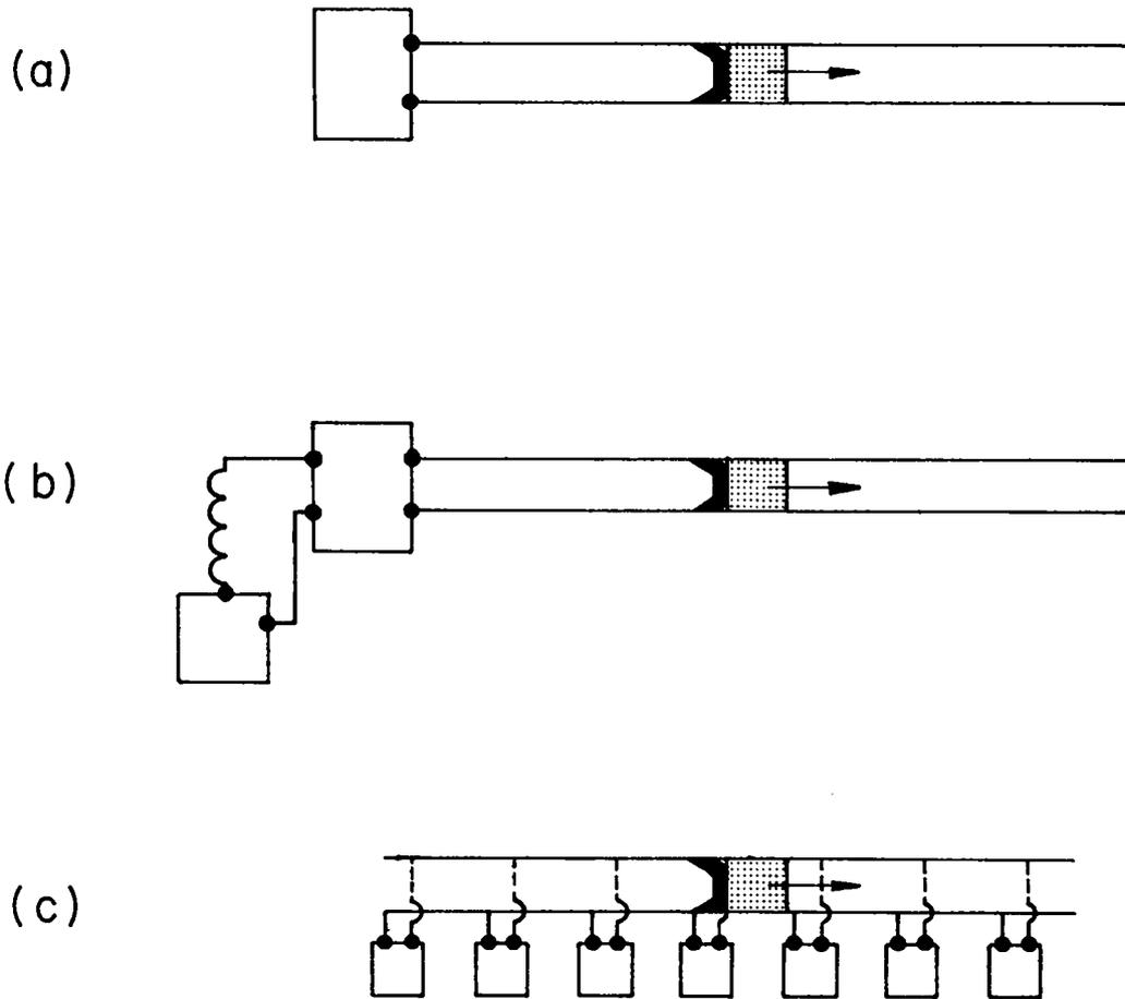
Figure 5: Schematic representations of three railgun-energy store systems with,
