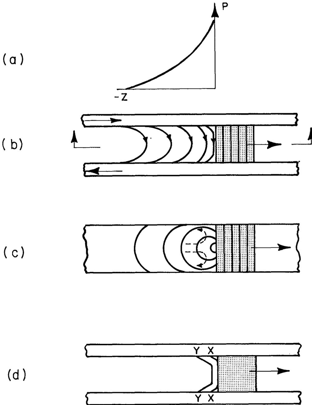
Figure 3: (a) Expected pressure on the centerline of railgun with plasma armature versus distance behind the projectile's driving face.
