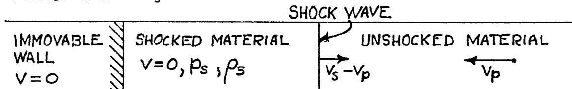
The equations applicable to the moving piston case apply equally here. In addition, in this system it is particularly easy to calculate the temperature of DT. Assume a cylinder of DT, containing  $N$  D+T atoms, impacts at velocity  $v_p$  against a hard wall. The initial kinetic energy is
