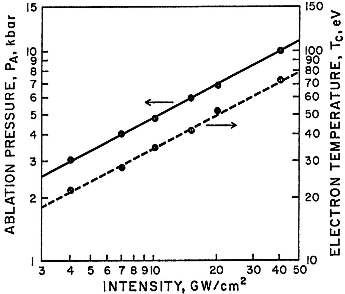
Fig 4 Ablation pressure and electron temperature at the absorption surface as a function of laser intensity. The laser wavelength,  $\lambda = 5\mu$ . The solid circles are time (0.5  $\mu$ sec) averaged results from the 1-D calculations.
