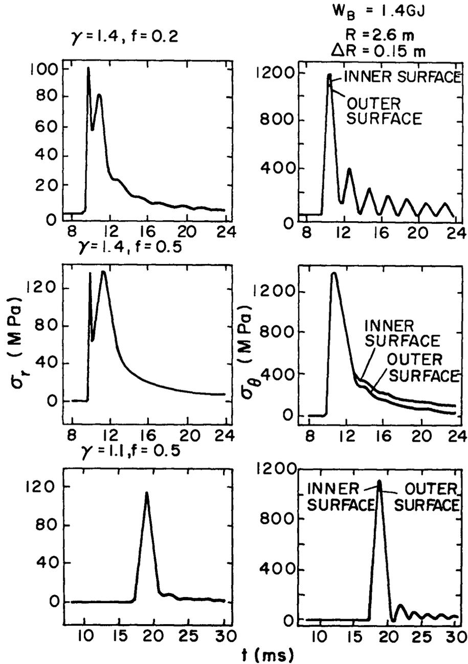
Fig. 7. Time-dependence of radial ( $\sigma_r$ ) and hoop ( $\sigma_\theta$ ) stress for a 1.4-GJ blast energy release to a  $M = 25$ -kg mass in a gas (He)/liquid (LiPb) mixture contained in a  $R = 2.6$ -m,  $\Delta R = 0.15$ -m spherical vessel that is initially pressurized to 0.1 MPa. The initial volume fraction of liquid is  $f$ , and  $\gamma$  is the heat capacity ratio for the gas.
