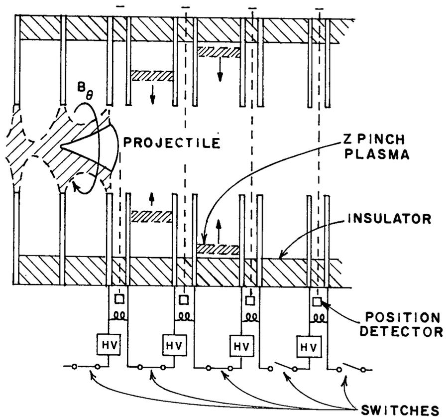
Fig. 5 Schematic diagram of a plasma-impulse accelerator<sup>(20)</sup>
