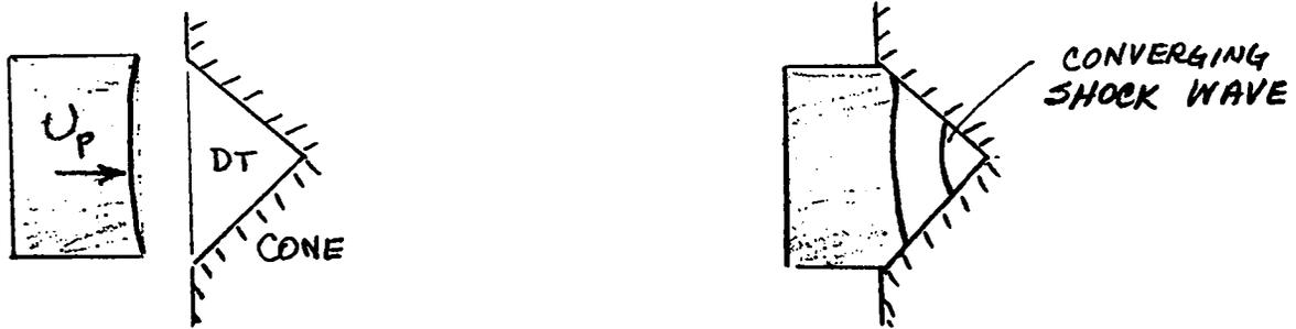
As the cone is part of a sphere, we have a segment of a spherical implosion. However, unless the wave is uniformly initiated, the wave will not focus as illustrated above. It tends to break up and behave as if it were plane with shock reflections at the walls, as shown on the left.
