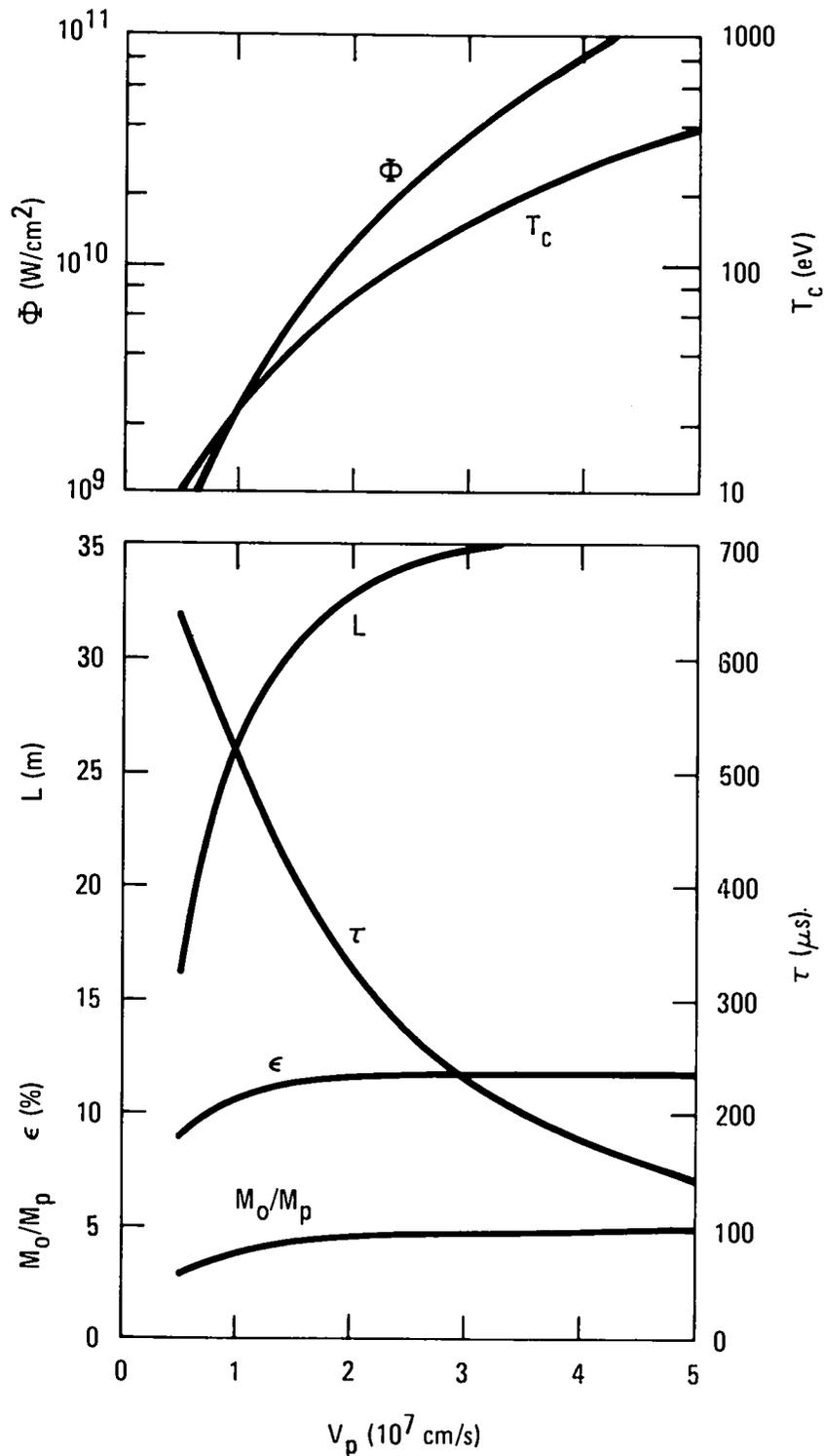
Fig. 5. Acceleration of hydrogen pellets by CO<sub>2</sub> lasers to velocity  $V_p$  at optimal efficiency. Curves show laser flux  $\Phi$ , temperature at critical surface  $T_c$ , efficiency  $\epsilon$ , and ratio of initial to final pellet mass  $M_0/M_p$  for any  $M_p$ . For  $M_p = 0.05$  g and compressed pellet density  $0.1$  g/cm<sup>3</sup>, curves show acceleration length  $L$  and time  $\tau$ .
