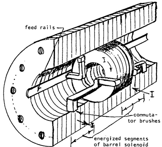
Fig. 3: The helical railgun.
