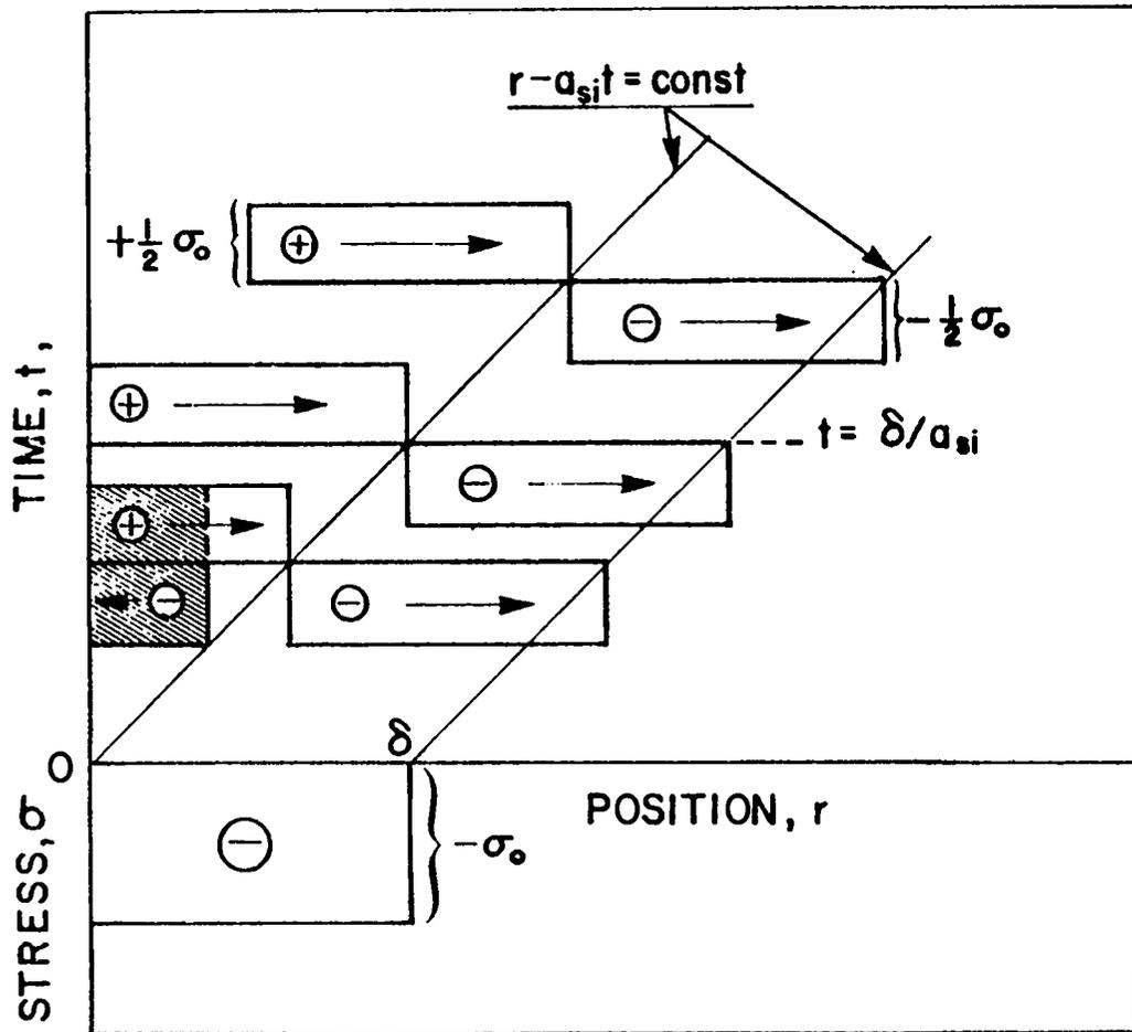
Fig. 7. Stress wave propagation (schematic) +: tensile, - compressive.
