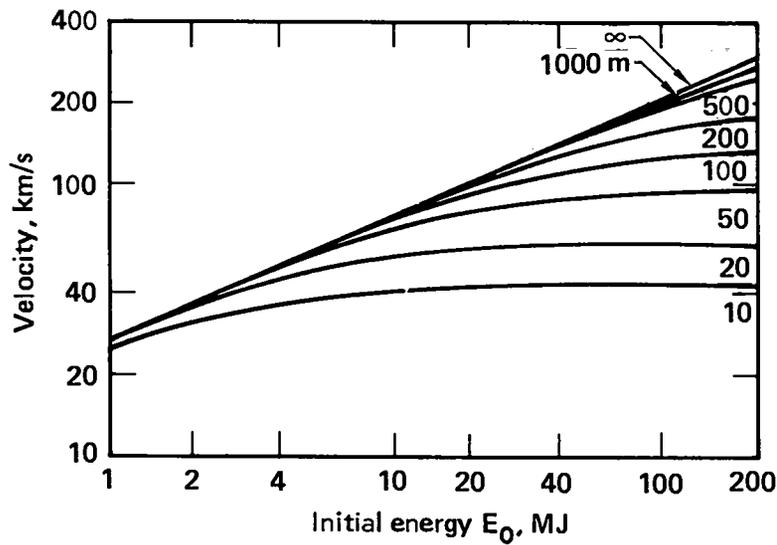
FIG. 2. Launch velocity versus initial energy stored in the inductor (for various accelerator lengths). Here,  $p = 40$  mm,  $w = h = 2\ell = 10$  mm,  $m_T = 1.23$  g (0.1-g payload),  $I_0 = 750$  kA (see Table 2).
