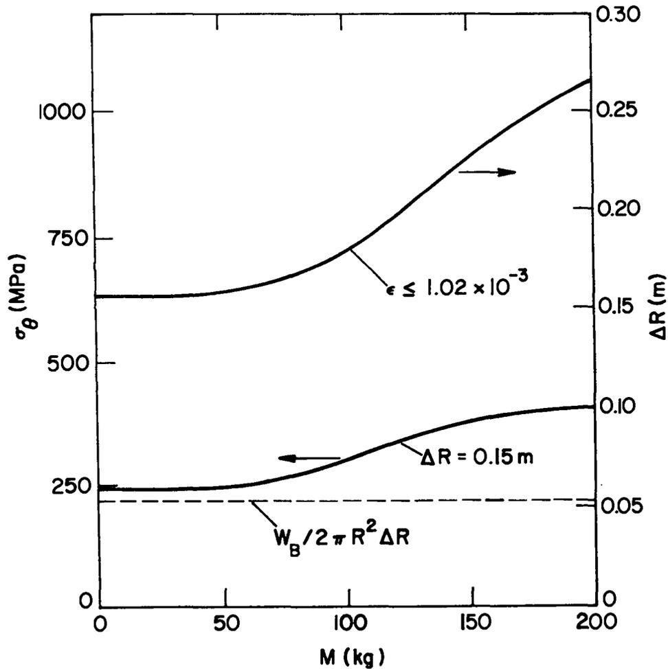
Fig. 6. Dependence of maximum hoop stress,  $\sigma_\theta$ , on mass  $M$  assigned to a vacuum release of 1.4-GJ energy for either fixed strain,  $\epsilon$ , or a fixed vessel thickness  $\Delta R$ . The vessel radius is  $R = 2.6 \text{ m}$ . Dashed line indicates virial theorem prediction, multiplied by 2 to account for shell oscillations, Eq. (20A).
