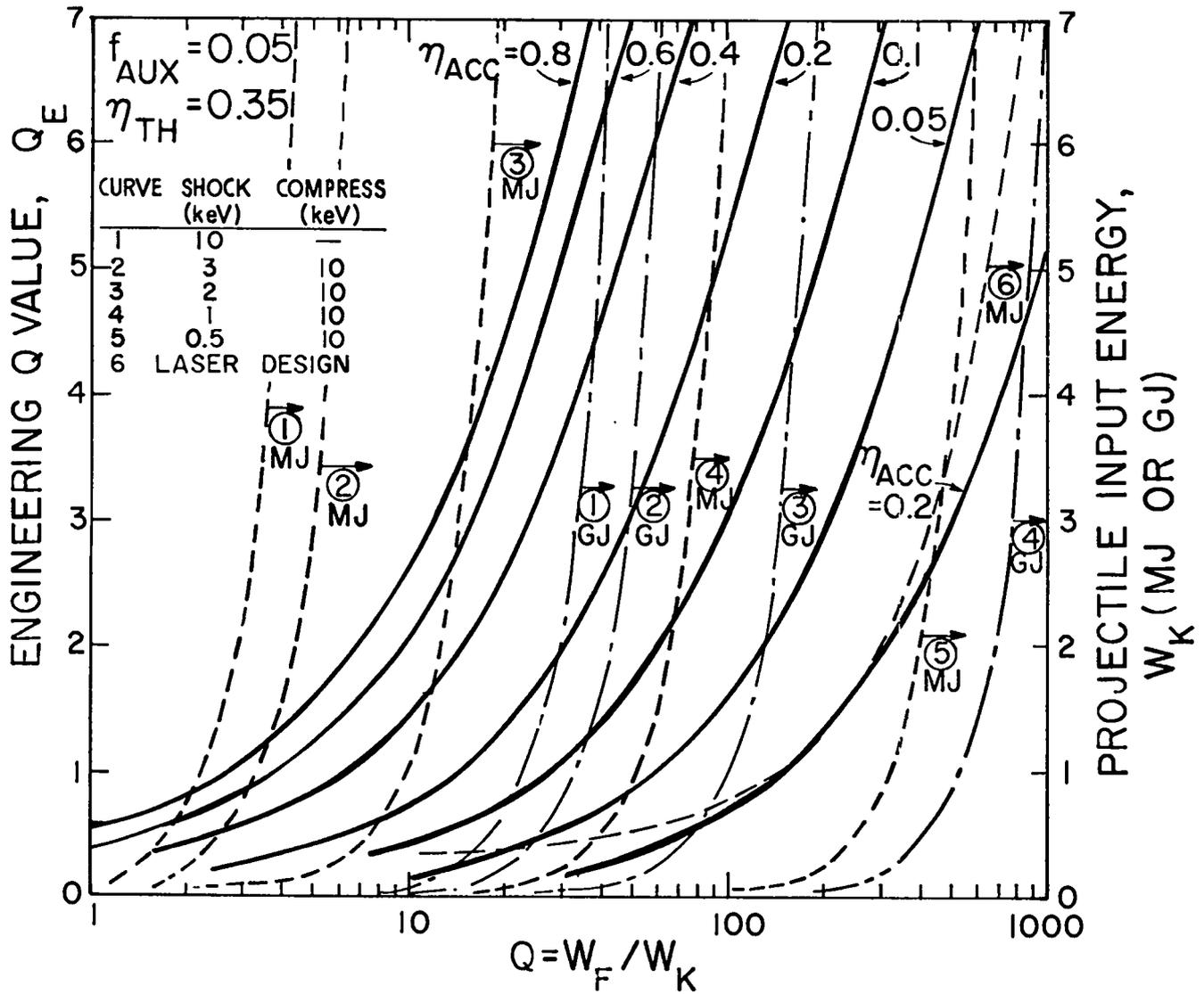
Fig.7 Parametric systems design curves for an Impact Fusion Reactor (IMF) showing limiting-case yield curves. Solid line curves represent  $Q_E$  versus  $Q$  and  $\eta_{ACC}$ , dashed-dot curves represent  $Q$  versus  $W_K$ (GJ) and the dashed curves represent  $Q$  versus  $W_K$ (MJ).
