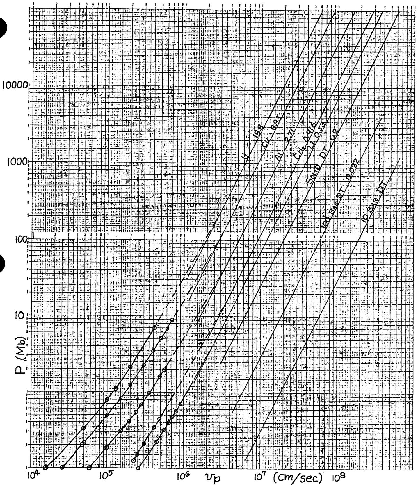
Fig. 1. Pressure vs. particle velocity Hugoniots for representative materials. Hugoniots are experimental below  $10^6$  cm/sec and 10 Mb. Straight lines at high velocity and pressure assume  $\gamma = 5/3$  gas law behavior.
