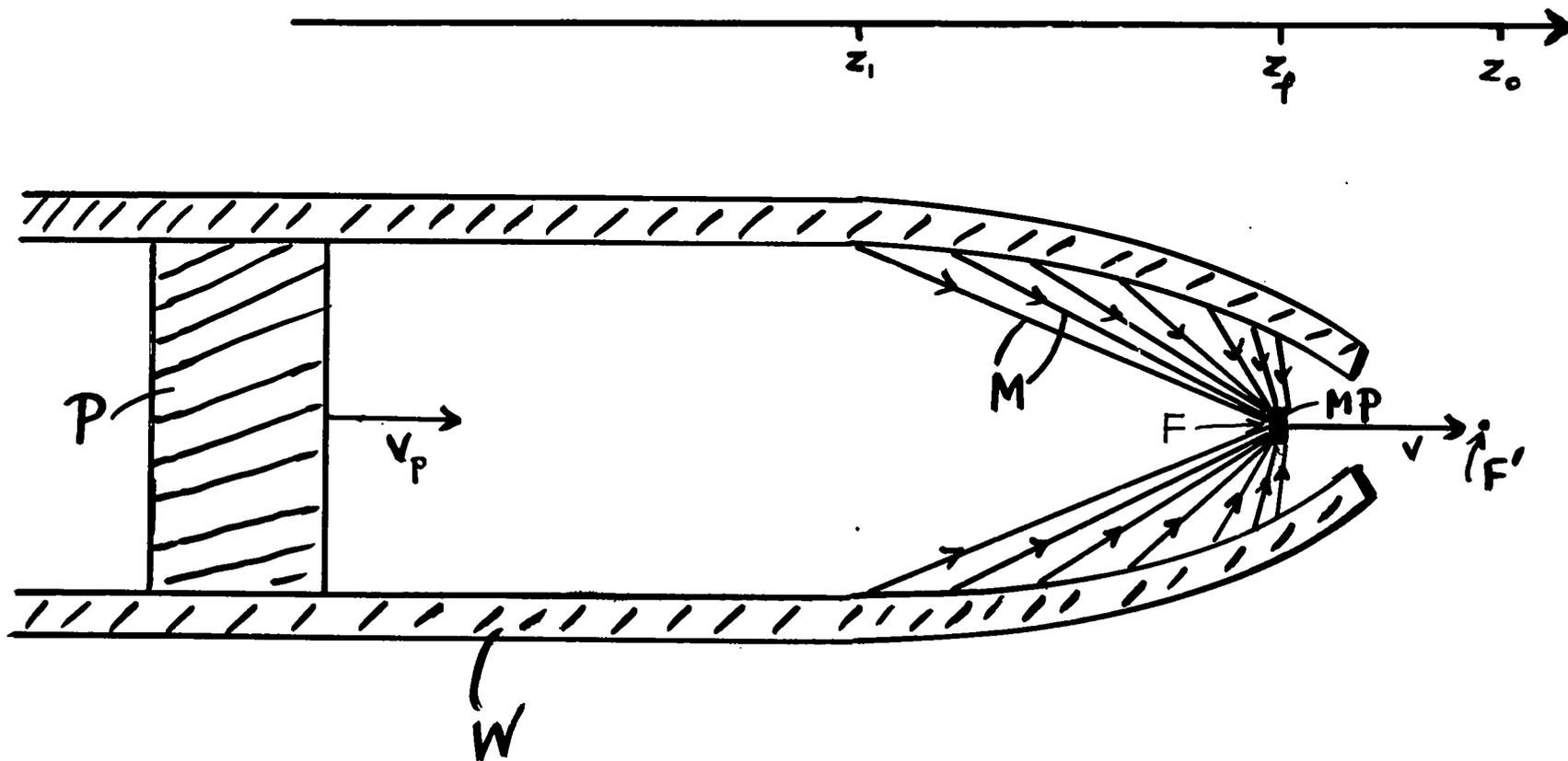
Fig. 1. P piston, W wall with concave curved end, M Mach lines in the  $r - z$  plane, MP macroparticle, F wave focus, F' virtual focus.
