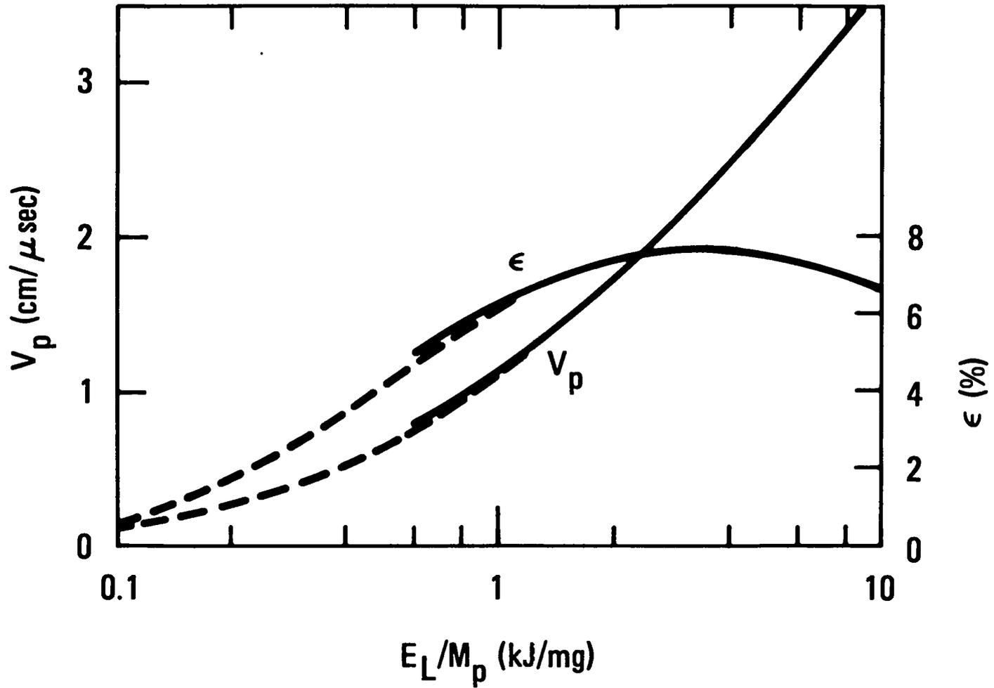
Fig. 2 Final hydrogen pellet velocity  $V_p$  and optimized efficiency of conversion of laser pulse energy to pellet kinetic energy  $\epsilon$  versus ratio of laser pulse energy to final pellet mass. Dashed curves represent less efficient acceleration at lower laser flux required to avoid pellet disassembly by shocks.
