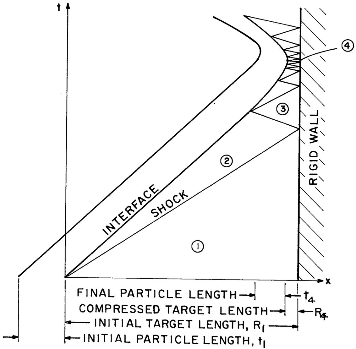
Figure 1. x-t Diagram of Wave Motion in Target.
