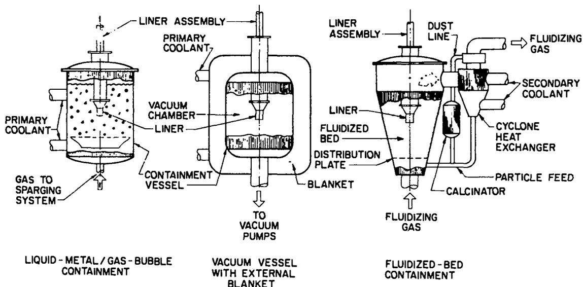
Fig. 2. Schematic diagrams of several blast containment and primary coolant schemes considered for the FLR.
