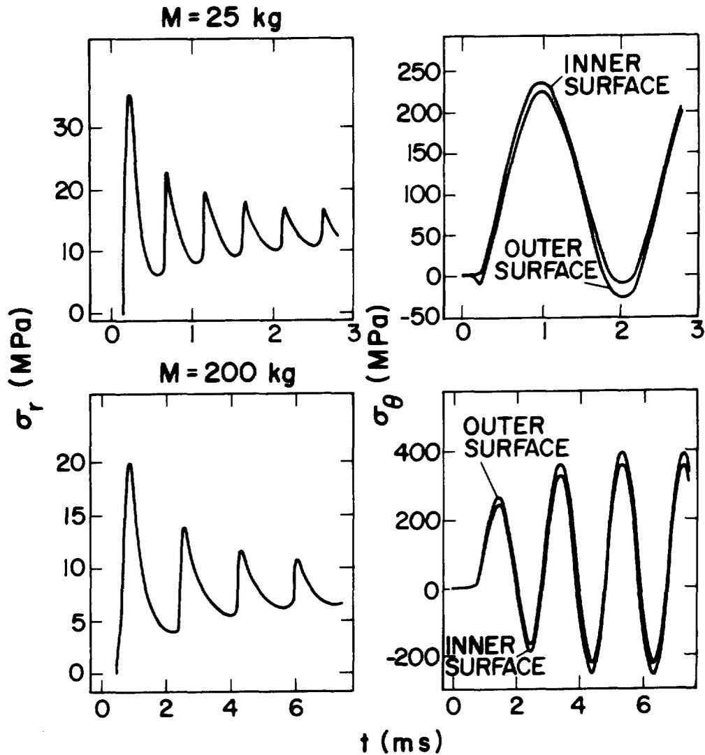
Fig. 5. Time dependence of radial ( $\sigma_r$ ) and hoop ( $\sigma_\theta$ ) stress for a vacuum energy release of 1.4 GJ in a spherical vessel of 2.6-m radius and 0.15-m wall thickness. The mass that contains this energy is  $M$ . These results can be scaled to other vessel dimensions ( $R, \Delta R$ ) by Eq. (20A).
