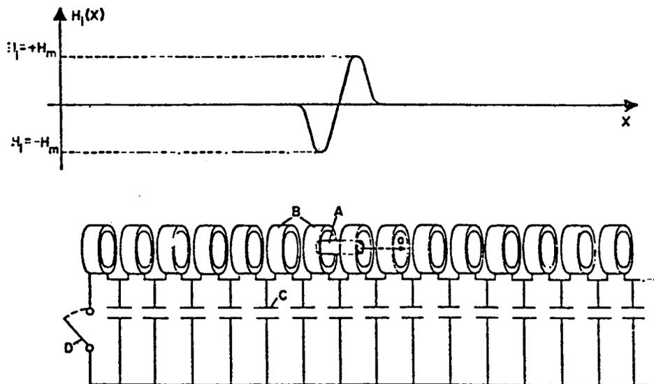
FIG. 5.—Transmission line accelerator. A: accelerated solenoid; B: field coils; C: capacitors; D: switch to be closed to start travelling magnetic wave.  $H_1(x)$ : magnetic field on transmission line relative to the frame of the solenoid.  $n(x)$ : windings per unit length in field coils (arbitrary units).
