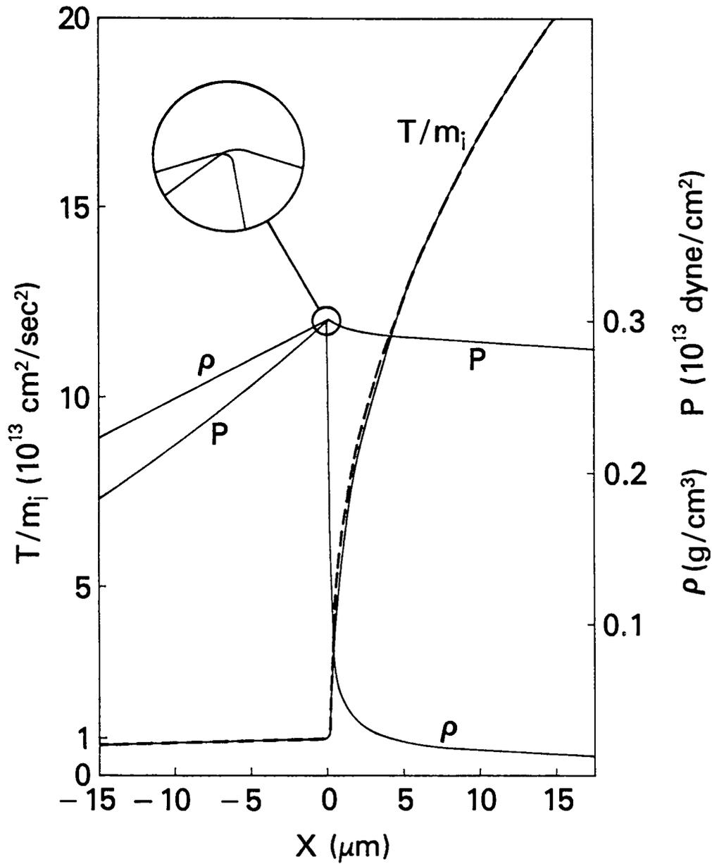
Fig. 3. Temperature, density, and pressure profiles at the ablation layer with  $T/m_i = 10^{13} \text{ cm}^2/\text{s}^2$ ,  $v = 2.2 \times 10^5 \text{ cm/s}$ , and  $\rho = 0.3 \text{ g/cm}^3$  specified at the surface of peak density, and acceleration  $g = 3 \times 10^{15} \text{ cm/s}^2$ . Dashed curve is analytic temperature approximation.
