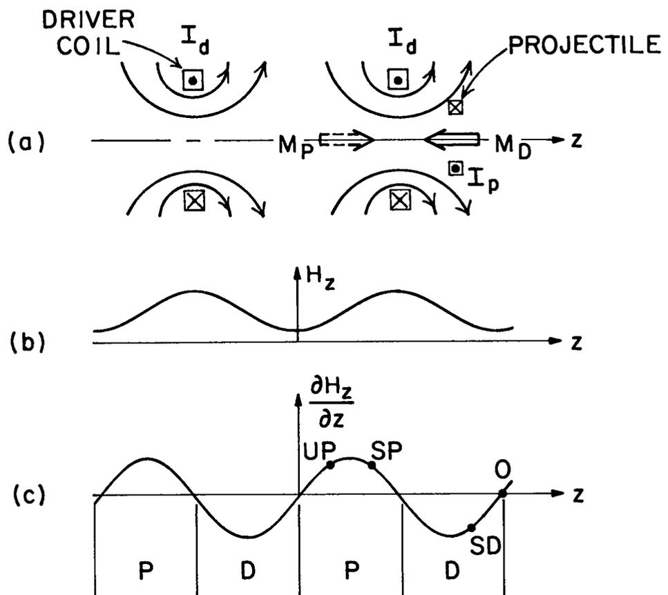
Fig. 4 Illustrating the magnetic fields and magnetic-moment  $M$  of driving coils(d) and superconducting projectile in a traveling-wave accelerator.
