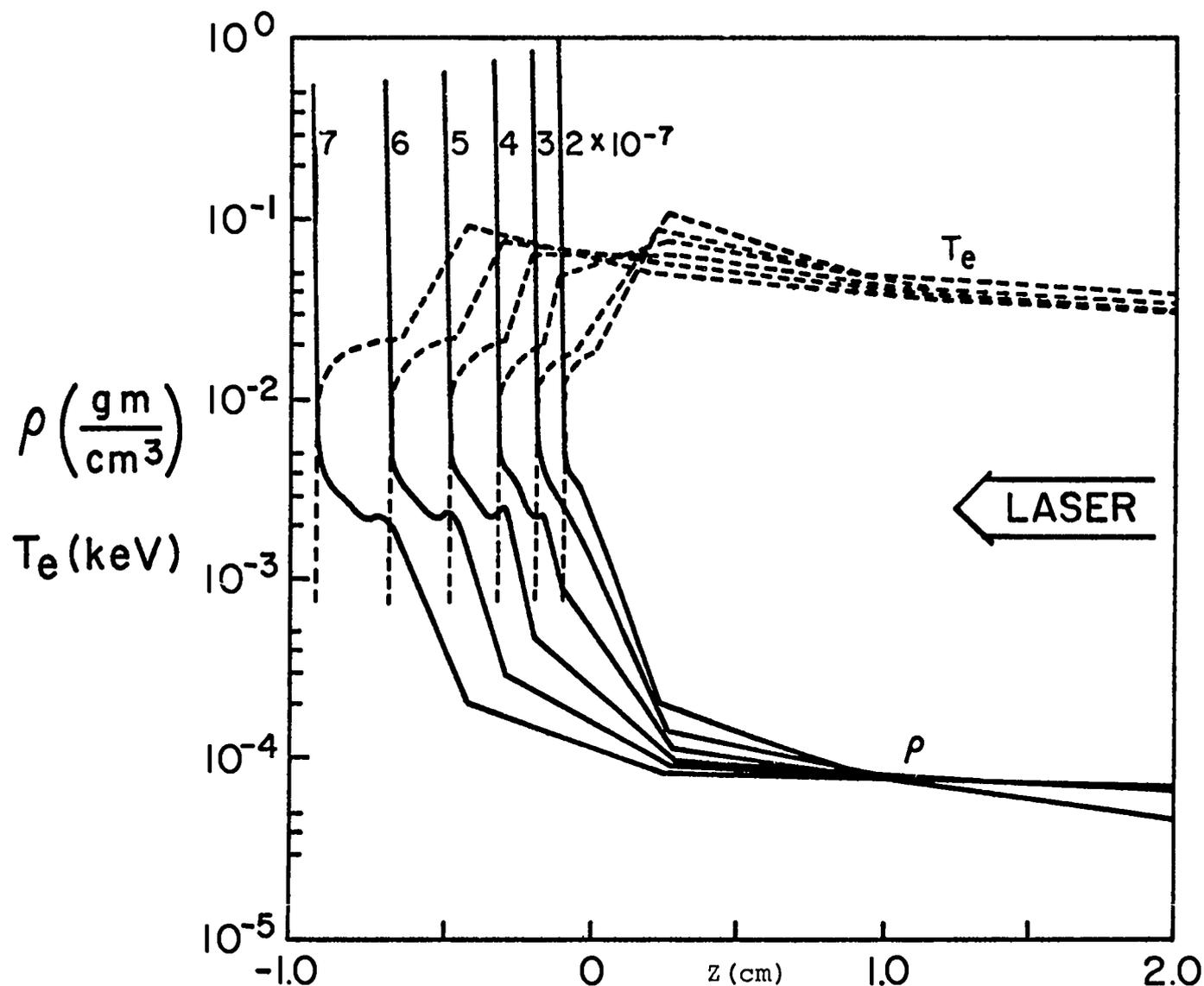
Fig. 3 Spatial profiles of electron temperature and plasma density at times of  $t = 0.2, 0.3, 0.4, 0.5, 0.6,$  and  $0.7 \mu\text{sec}$  after the laser is switched on. Results from a 1-D calculation with  $I = 4 \times 10^{10} \text{ W/cm}^2$ , laser wavelength,  $\lambda = 5 \mu$ , and a glass ( $\text{SiO}_2$ ) BB.
