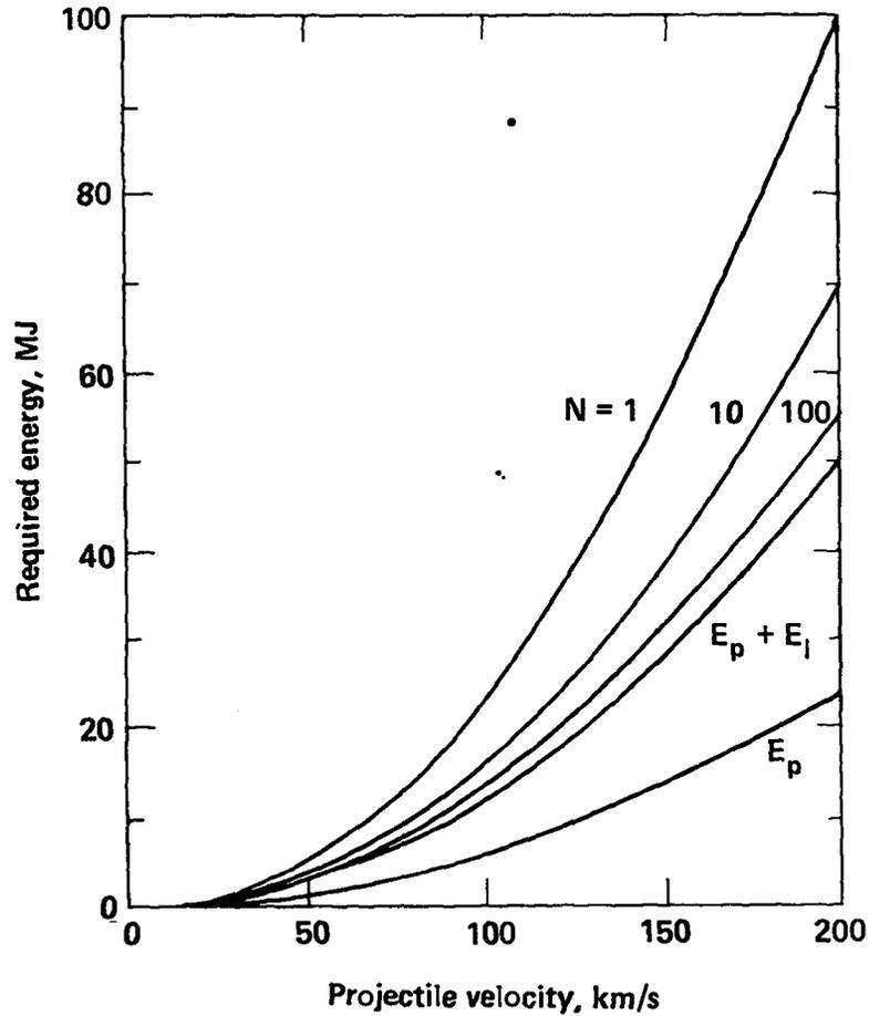
FIG. 5. Required energy versus projectile velocity for 1-, 10-, and 100-section railguns (projectile mass 1.23 g, initial current of each section 750 kA,  $p = 40$  mm).
