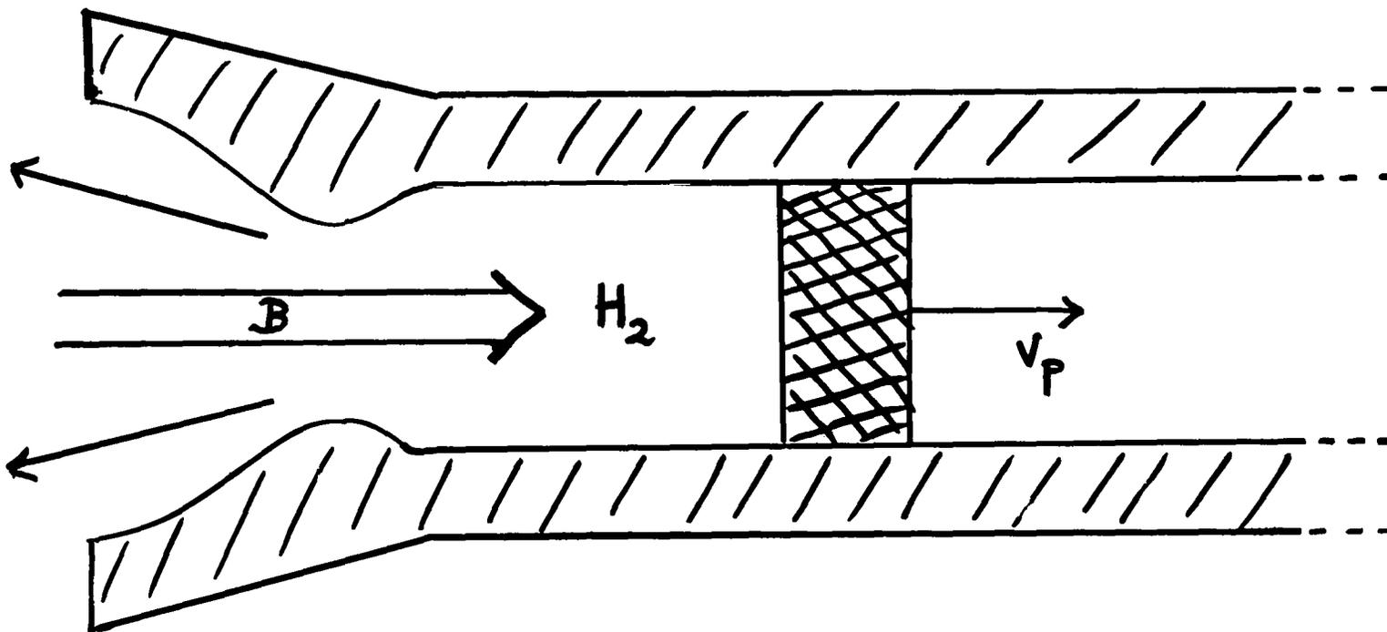
Fig. 4. Propulsion of piston by recoilless rifle using a hydrogen propellant and drawing its energy from an intense charged particle beam B.
