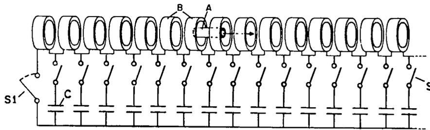
Fig. 3 Schematic diagram of a traveling-wave accelerator<sup>(12)</sup>
