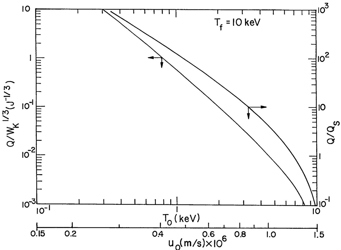
Fig. 8 Range of possible yield curves ( $Q$  versus  $W_K^{1/3}$ ) for a lossless adiabatic compression as a function of initial projectile (DT/tamper) velocity or initial shock-preheat temperature. Dependence of associated  $Q$ -value relative to purely shock-heated case ( $Q_s$ ) is also shown. Note that  $Q$  is an incremental value relative to  $Q_s$ .
