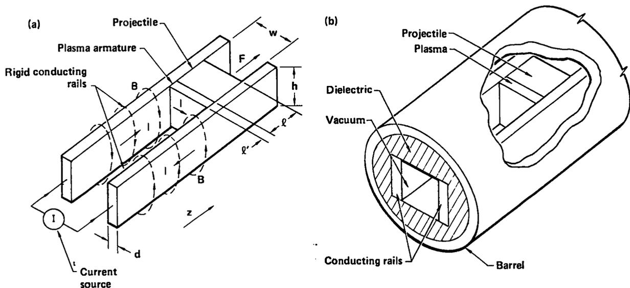
FIG. 1. Sketches of railgun. (a) Railgun accelerator. (b) Railgun assembly. The dielectric maintains the rail position and, along with the rails, confines the plasma behind the projectile.
