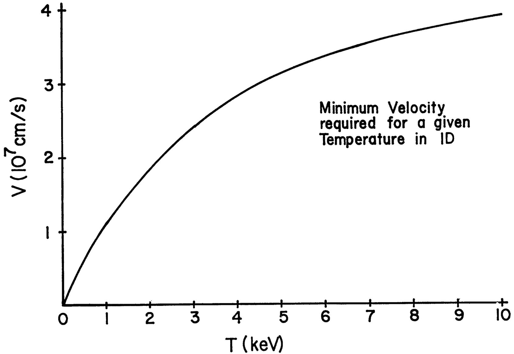
Fig. 1. Minimum impact velocity in ID needed to achieve a given temperature.
