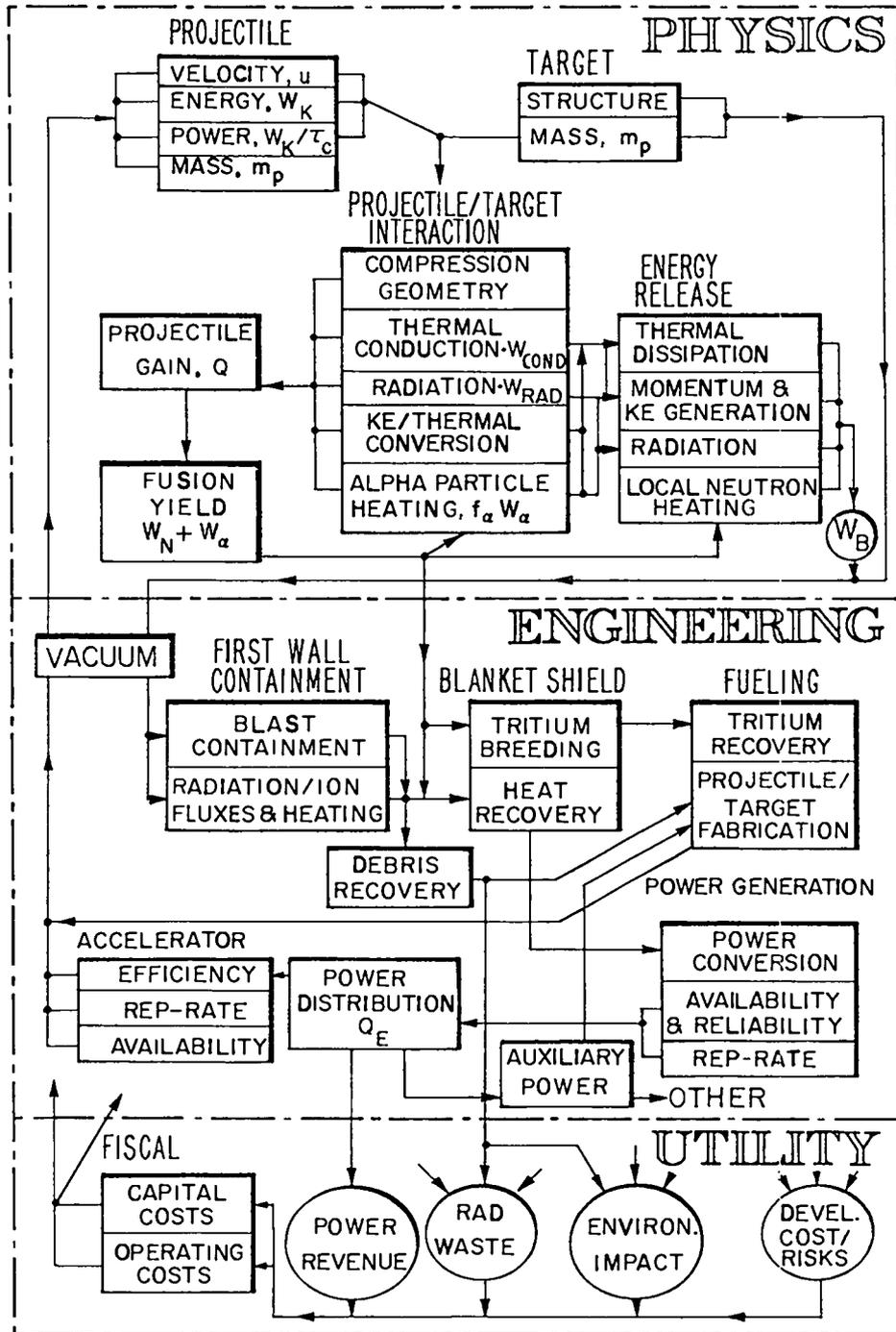
Fig. 3 Systems interfaces for an Impact Fusion Reactor (IFR).
