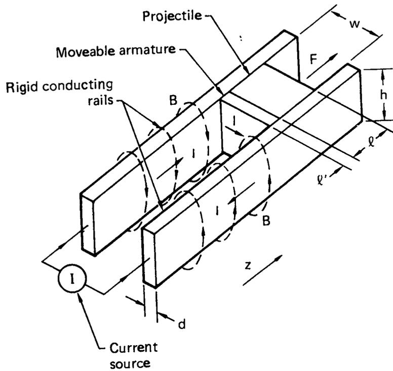
Fig. 1 Schematic diagram of a rail gun<sup>(11)</sup>
