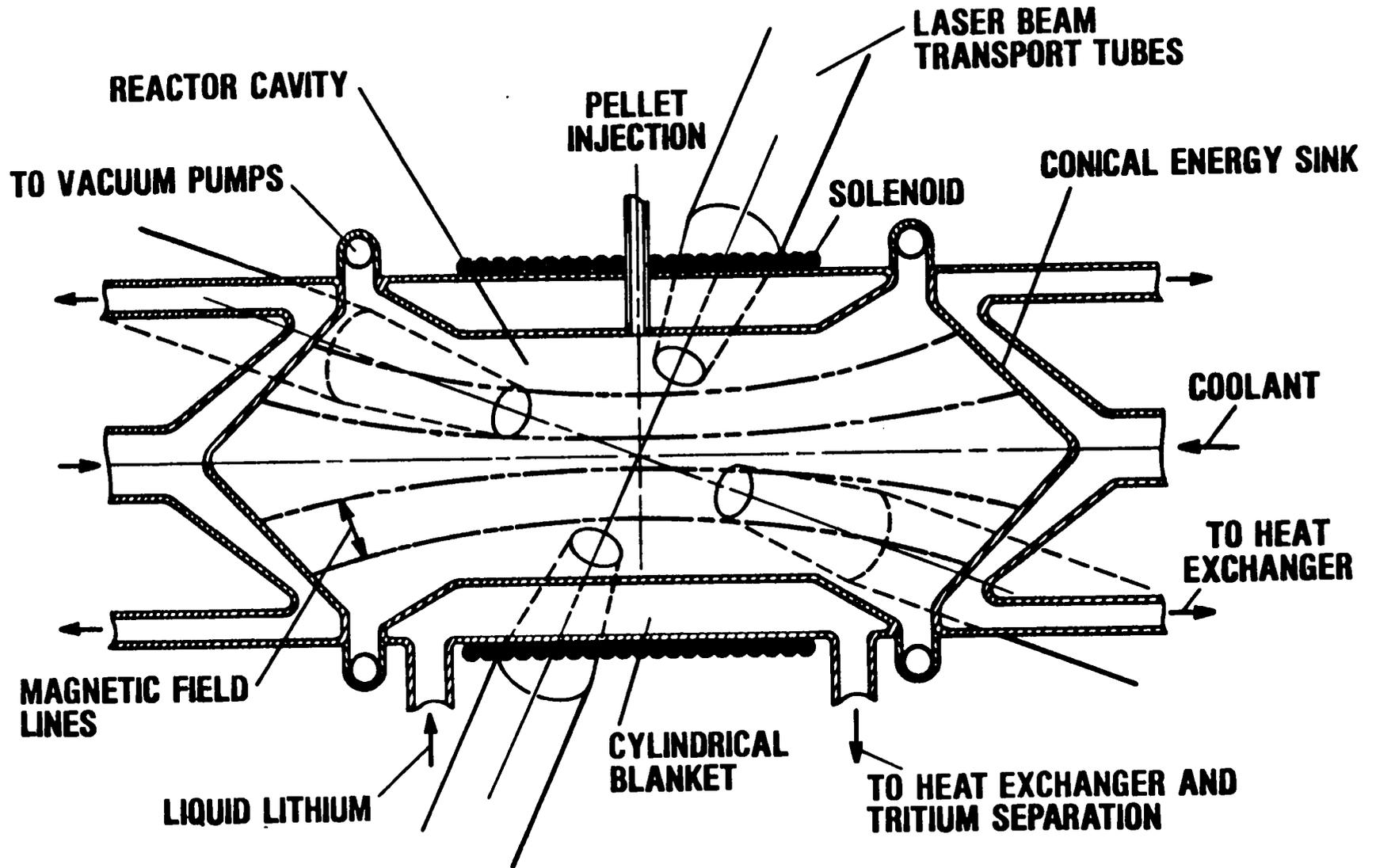
Fig. 4. The magnetically protected reactor concept.
