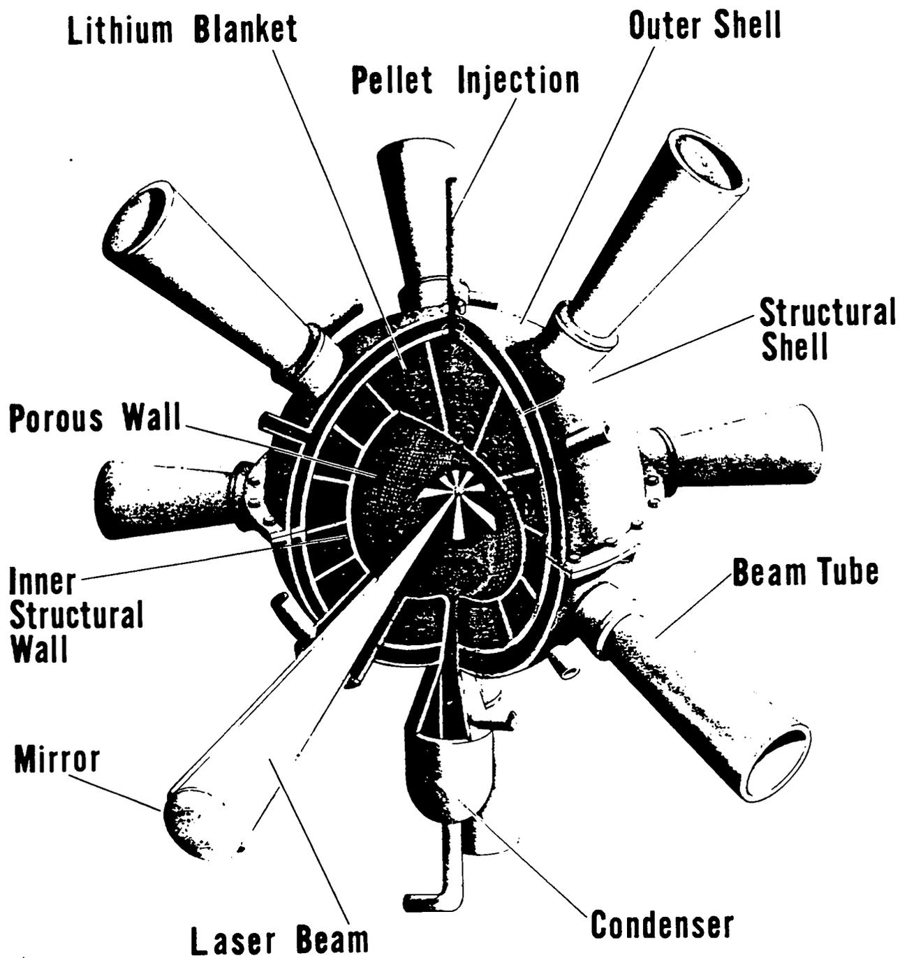
Fig. 3. The wetted-wall reactor concept
