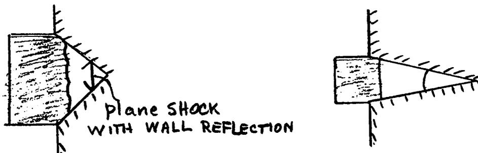
A situation which is probably less sensitive to the initial conditions is shown on the right with a smaller cone angle. However, such a situation has poorer surface to volume characteristics and thus increased losses.
