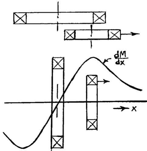
Fig. 1: The mutual inductance gradient as a function of drive coil position for planar and axial mass drivers; ref. 6.
