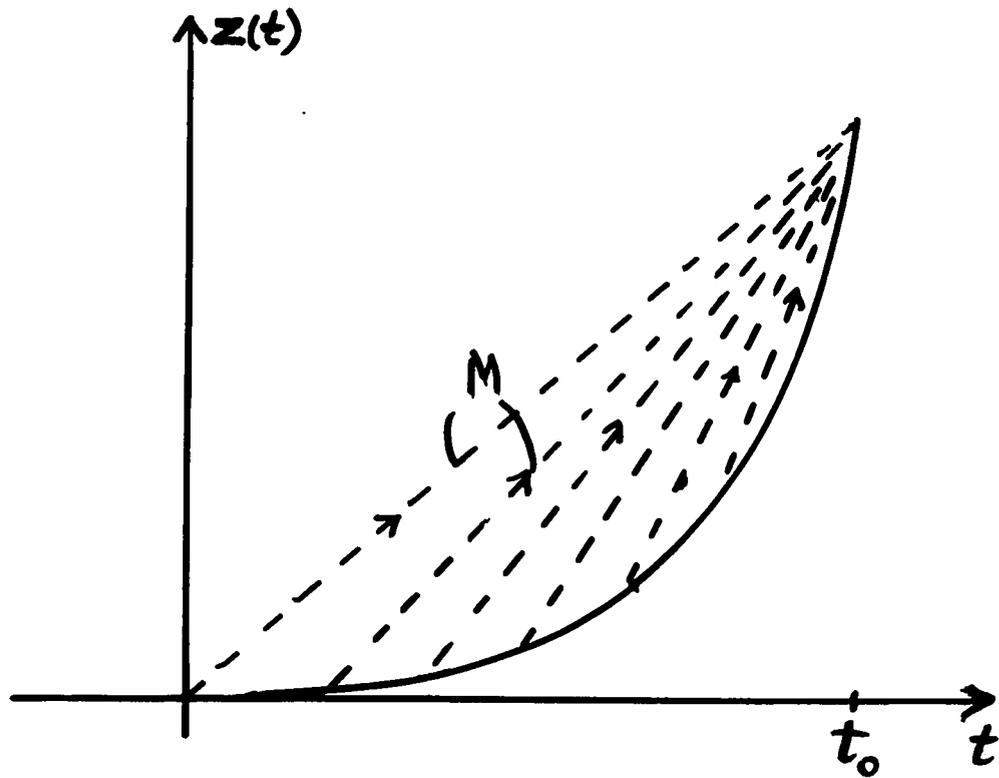
Fig. 2. Isentropic wave coalescence in time by accelerated piston: piston position  $z = z(t)$ ,  $M$  Mach lines in the  $z - t$  plane.
