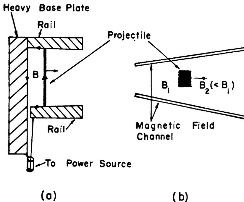
Fig. 1. Schematic drawings of projectiles accelerated by (a) magnetic fields and (b) magnetic field gradients.
