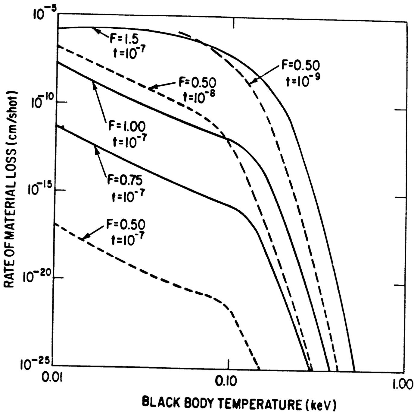
Fig. 1 Rate of material loss of carbon surface from x rays. F is fluence in J/cm<sup>2</sup>, t is pulse width in seconds.
