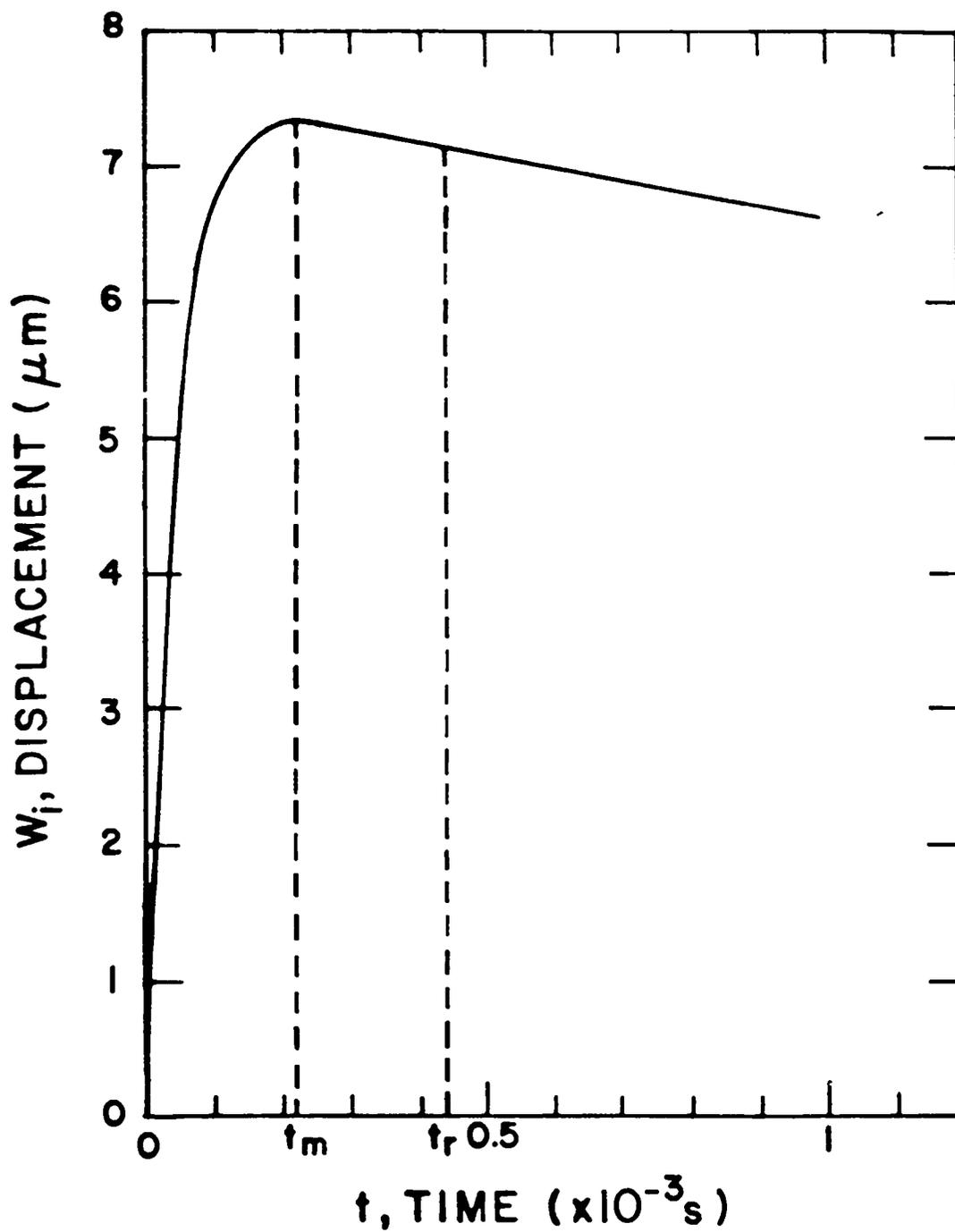
Fig. 6. Response of a structural shell in the presence of hydrodynamic coupling.
