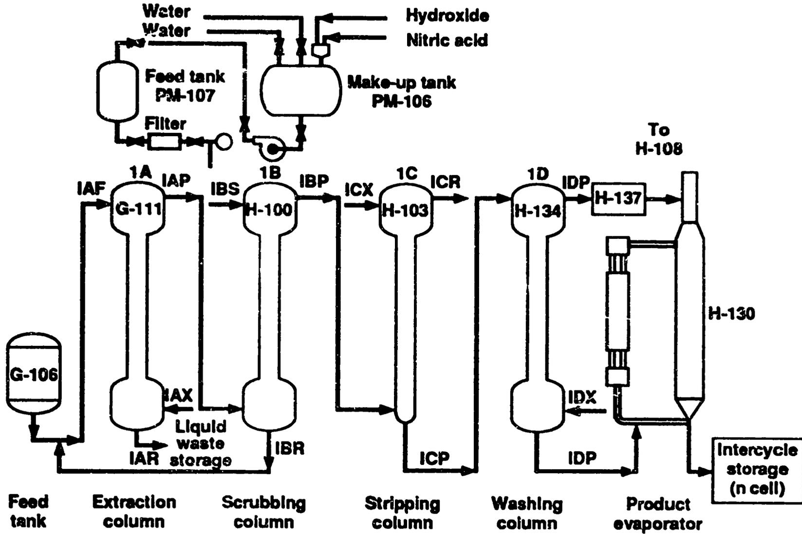
Figure 8. First-cycle extraction line, Idaho Chemical Processing Plant.
