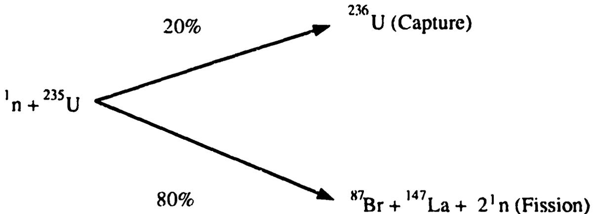
Figure 5. Neutron interaction with uranium.
