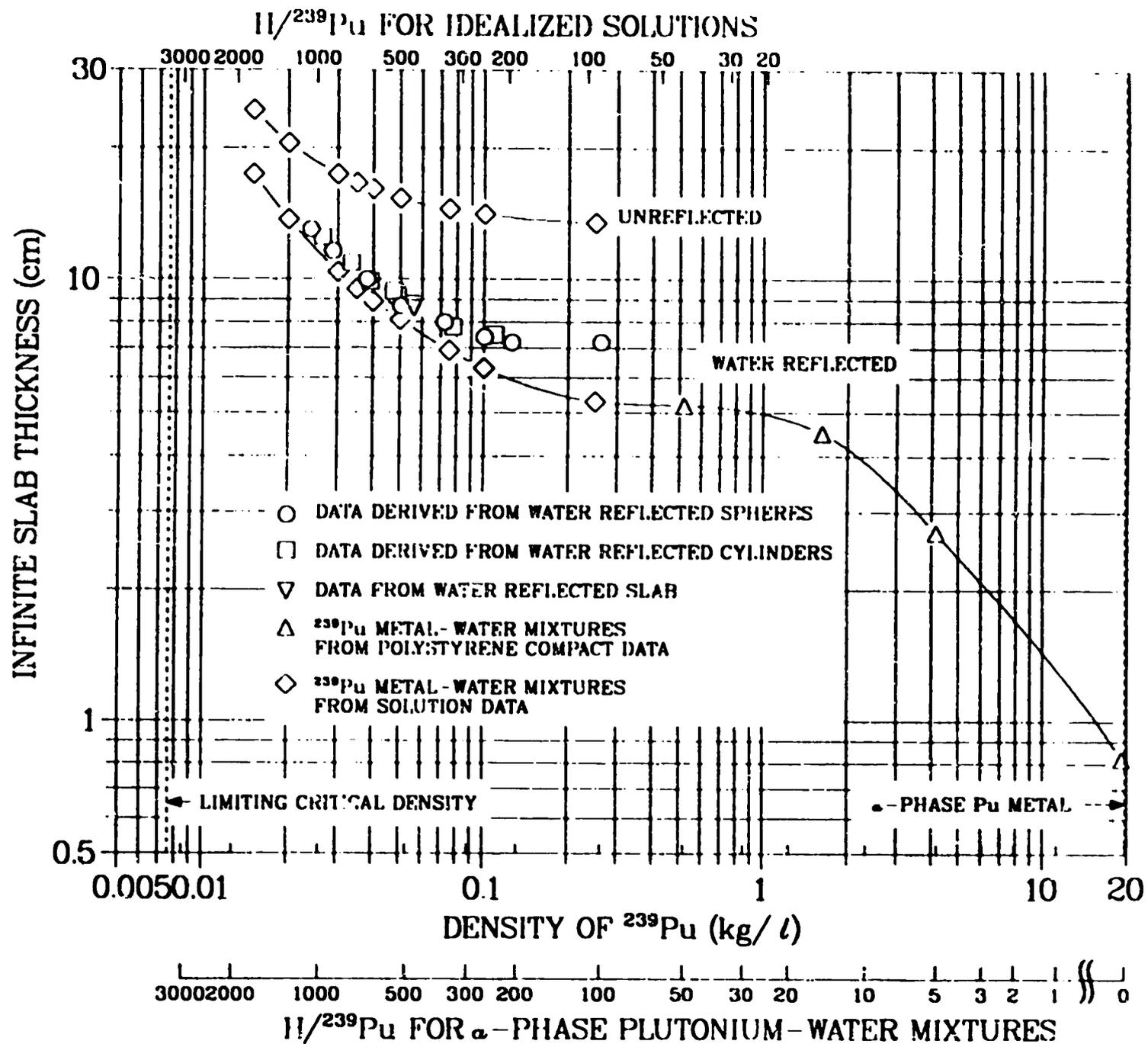
Figure 16. Estimated critical thicknesses of slabs, infinite in other dimensions, of homogenous water-moderated  $^{239}\text{Pu}$ . Unreflected infinite slabs are fictitious. The points suggesting an intermediate curve apply to water-reflected  $\text{Pu}(\text{NO}_3)_4$  solutions with 1 N  $\text{HNO}_3$  and 3.1%  $^{239}\text{Pu}$  content of the plutonium. (From LA-10860-MS, Figure 34).
