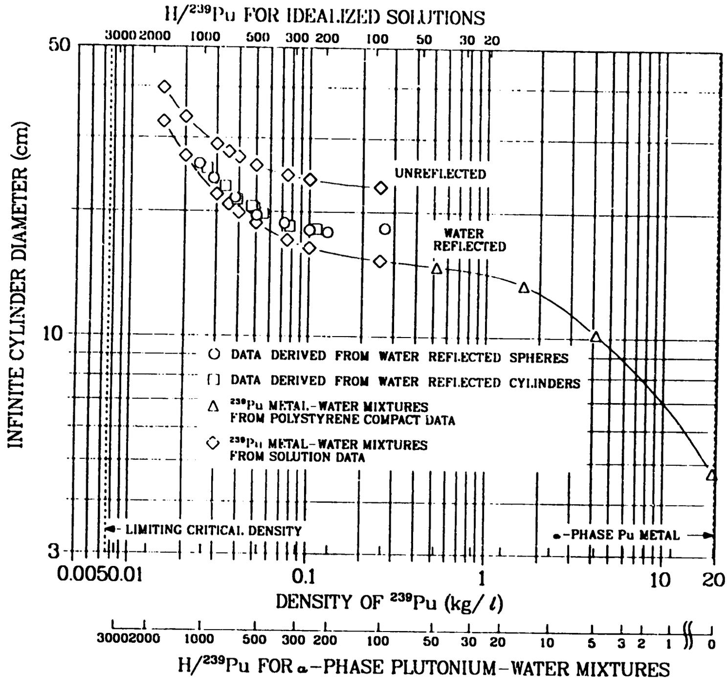
Figure 14. Estimated critical diameters of infinitely long cylinders of homogeneous water-moderated  $^{239}\text{Pu}$ . The points suggesting an intermediate curve apply to water-reflected  $\text{Pu}(\text{NO}_3)_4$  solutions with 1 N  $\text{HNO}_3$  and 3.1%  $^{240}\text{Pu}$  content of the plutonium. (From LA-10860-MS, Figure 33).
