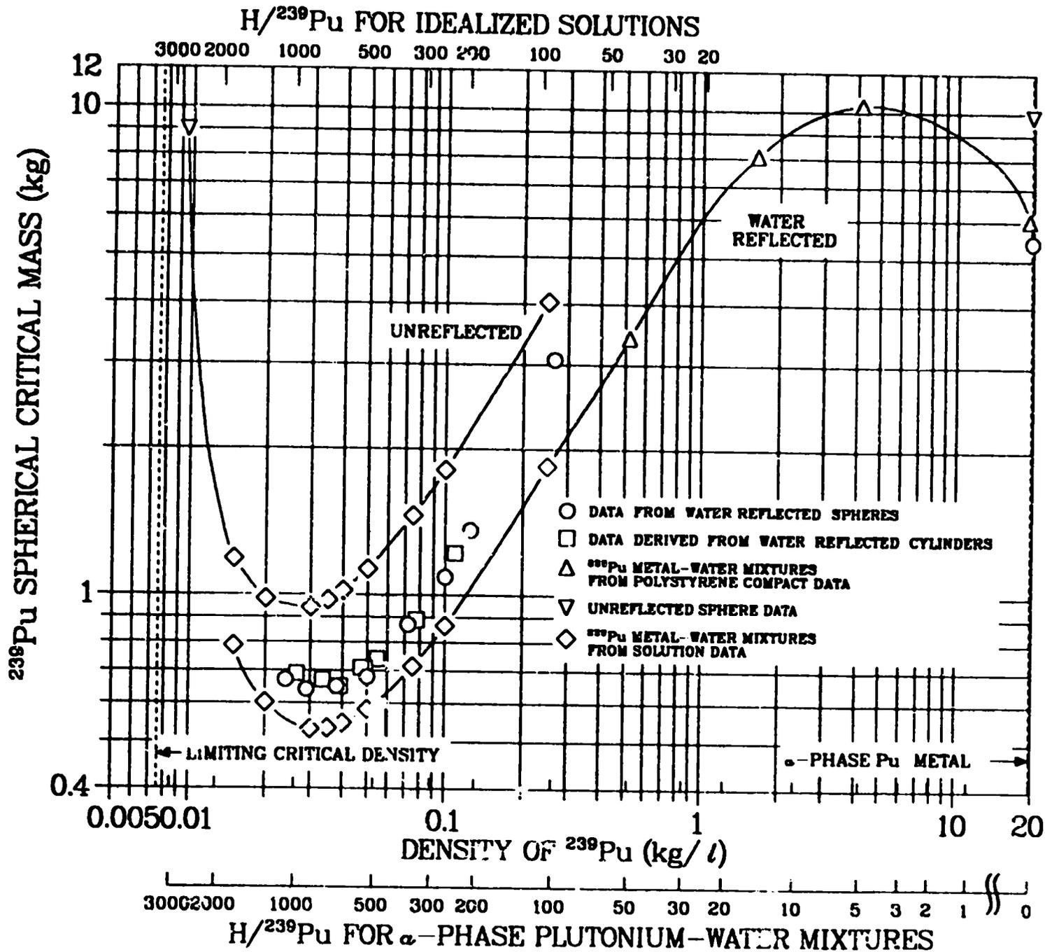
**Figure 11. Critical masses of homogeneous water-moderated <sup>239</sup>Pu spheres. The points suggesting an intermediate curve apply to water-reflected Pu(NO<sub>3</sub>)<sub>4</sub> solutions with 1 N HNO<sub>3</sub> and 3.1% <sup>240</sup>Pu content of the plutonium. (From LA-10860-MS, Figure 31).**
