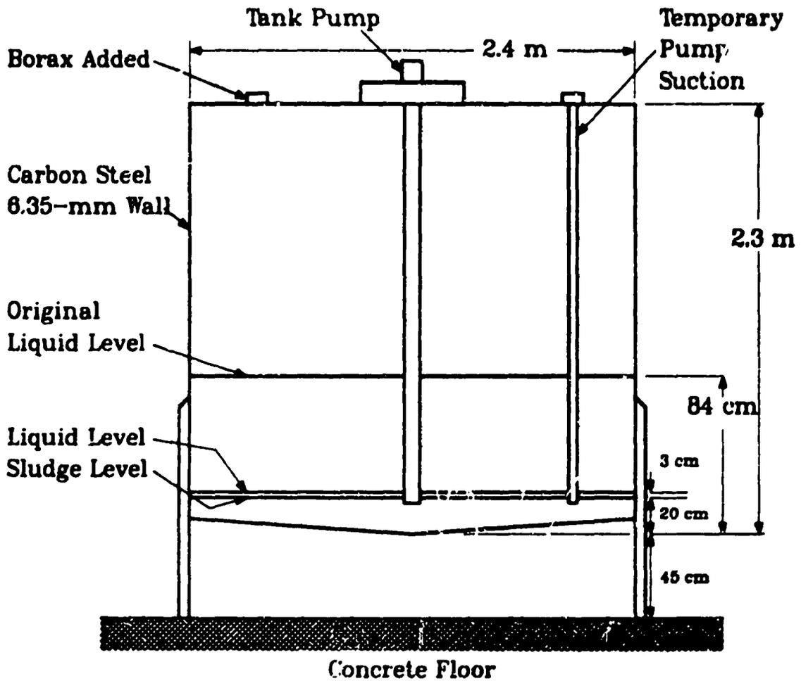
Figure 2. Caustic waste holding tank
