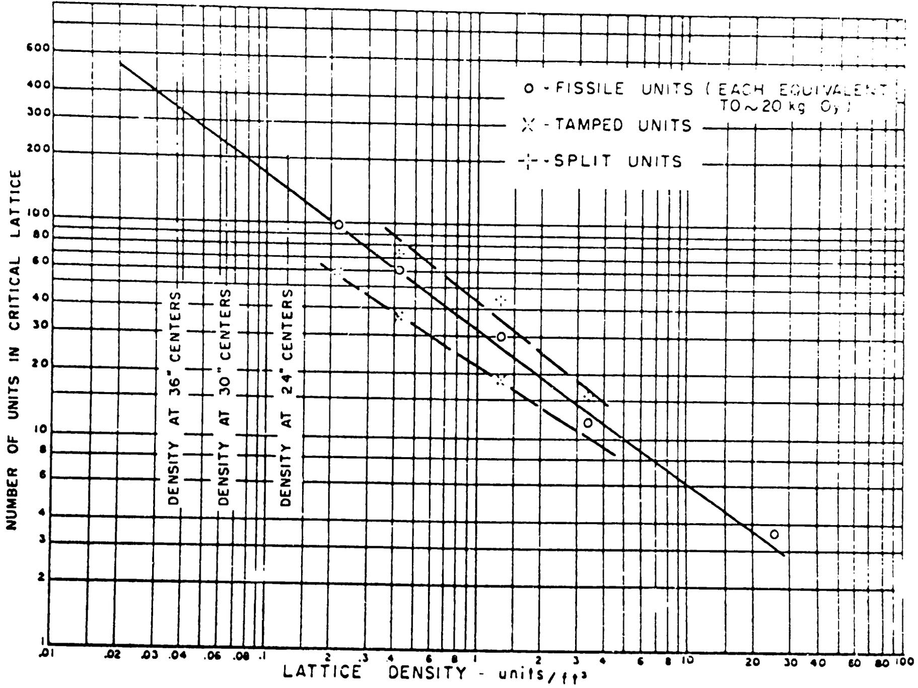
Figure 4. Attempt at generalization of vault test results.
