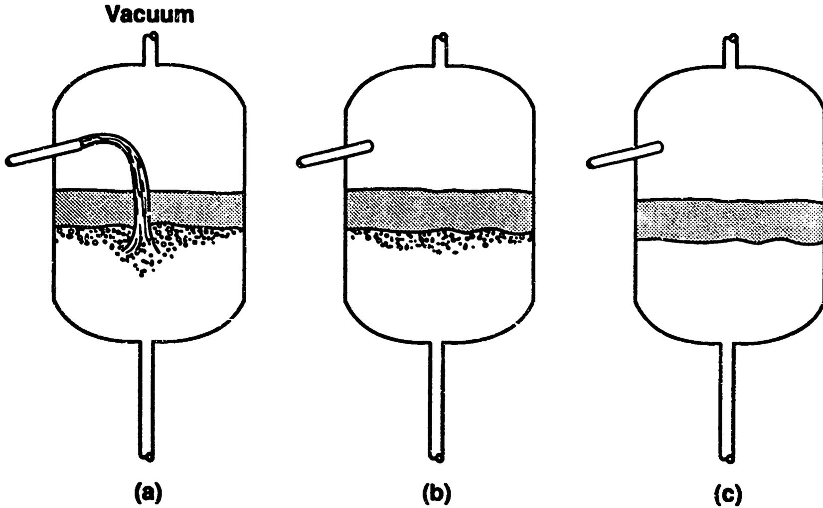
Figure 6. Solution transfer in the Windscale process line.
