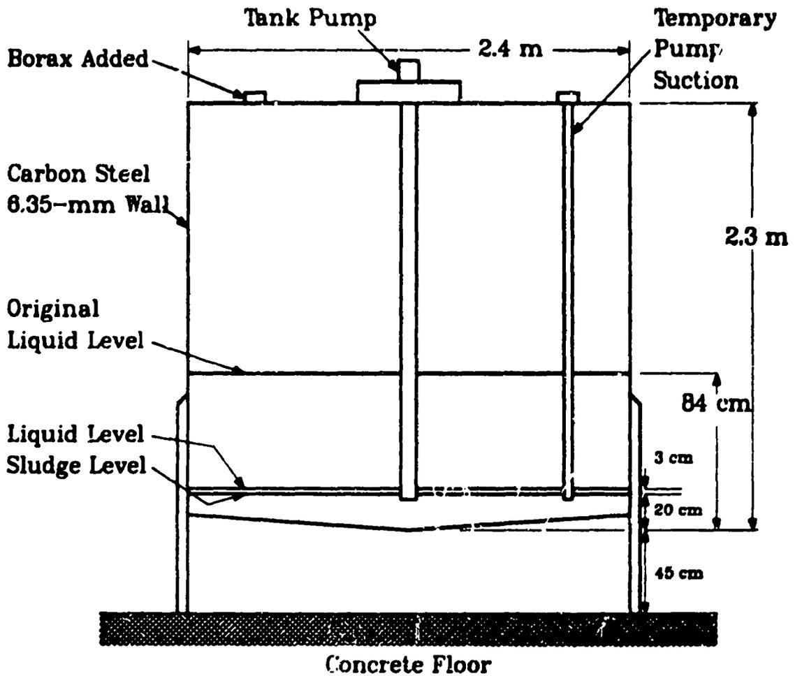
Figure 2. Caustic waste holding tank
