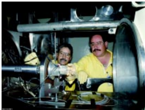
Ben Jacquez of Structure/Property Relations (MST-8), left, and Johnny Montoya of Nuclear Materials Technology (NMT-16) make adjustments to the target of the 40mm Launcher during its shakedown period in November 1995, before the windows and gloves were installed in the glove box. Researchers performed several experiments on inert samples this way to test the system before going hot. Part of the gun barrel is shown on the left; the round aluminum plate with the plastic cylinders is the target.
