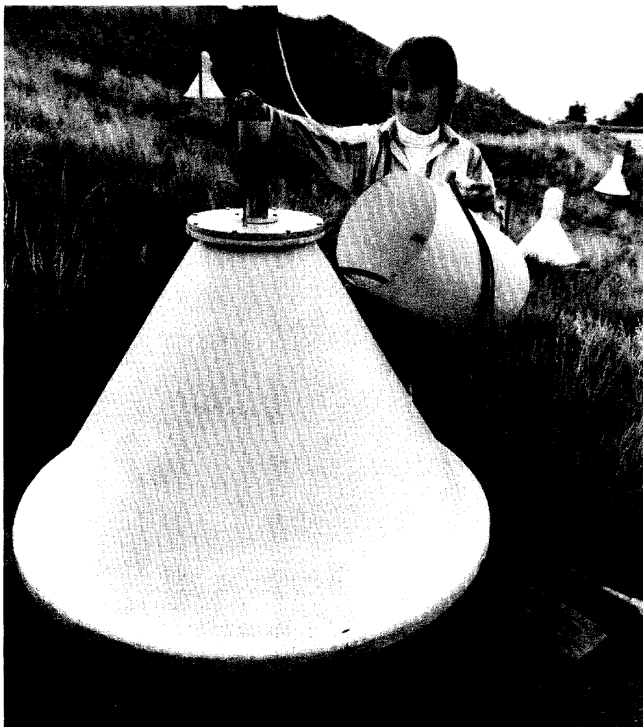
Fig. 10. Brenda Dingus, a University of Maryland graduate student, examining one of seventy scintillation counters being installed on the grounds of the Los Alamos Meson Physics Facility. The counters compose one element of an experiment aimed at resolving a current controversy about Cygnus X-3. (The experiment is a collaborative effort by the University of Maryland, the University of New Mexico, the University of California, Irvine, and Los Alamos National Laboratory.) The counters are distributed uniformly within a 60-meter-radius circle centered on the other essential element of the experiment—a spark-chamber detector already in use in a study of the scattering of accelerator-produced neutrinos by electrons. The array of scintillation counters will provide highly accurate data about the direction of the air showers detected and thus permit selection of air showers initiated by electrically neutral primaries from Cygnus X-3; the spark-chamber detector will provide data about the muon content of those same air showers. If the muon content of the selected air showers is inconsistent with that theoretically predicted for gamma-ray-initiated air showers, then either the theories of nuclear interactions need modification or some as yet undiscovered neutral particle is originating from Cygnus X-3.
