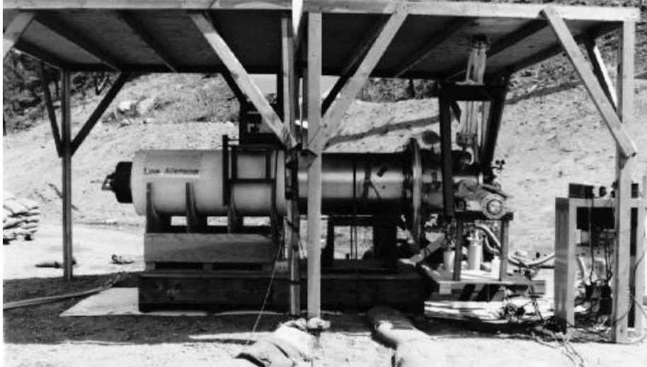
Figure 2. The Procyon High-Explosives Pulsed-Power System
