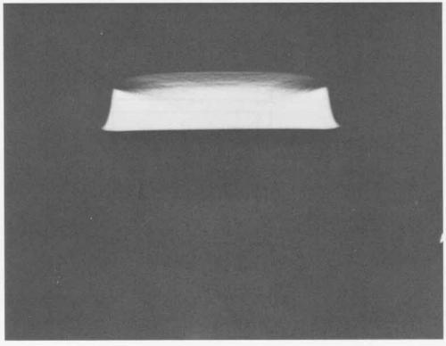
SHOT 796: Spherically Diverging Composition B-3 Detonation
