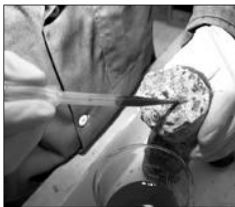
George Guthrie, one of the developers of ASR Detect, stains a concrete sample with a nontoxic solution that will detect the presence of the alkali-silica reaction (ASR) that degrades concrete.
