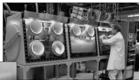
The Palladium Membrane Reactor with its heater and insulation is seen in the middle glovebox window. Inset shows the reactor's active components.
