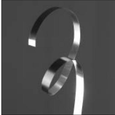
IBAD, aligns the cubic zirconia crystals at a specific angle. A superconducting ceramic, yttrium-barium-copper-oxide, is deposited by pulsed laser on top of the cubic zirconia layer. The precise orientation of the layers obtained through the IBAD process is necessary for superconducting materials if they are to allow high current to flow through them.
