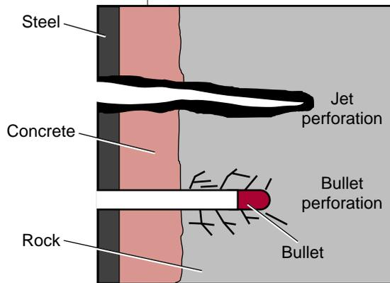
charges produce comparatively deep holes of about a foot that are lined with crushed rock of poor permeability, while bullets produce shorter holes surrounded by a desirable zone of cracked, uncrushed rock. In laboratory tests, the Los Alamos projectile launcher, which combines the best attributes of both the explosive and bullet devices, has produced deeper bullet penetrations that are surrounded by cracked rock. These
