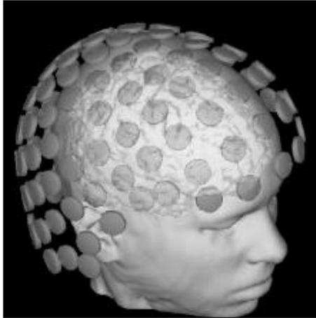
The Los Alamos researchers decided to take advantage of superconducting materials to improve upon the two-coil gradiometer. Because magnetic fields cannot penetrate superconductors, the Los Alamos biomagnetometer replaces the gradiometer's second coil with a superconducting surface shaped to surround the head like a helmet.
