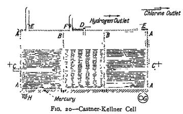
mercury to the negative electrode in the centre compartment.
