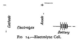
Liquids which, under the influence of the electric rrent, behave in the manner of the above are termed Electrolytes," and the process whereby they are split is called "Electrolysis". The laws relating to this decomposition of liquids by the electric current were enunciated by Faraday as follows:—
