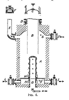
L is the main air inlet, while a secondary supply of air takes place through the vertical pipe G, the purpose of this latter air inlet being to ensure a thorough supply of air to all parts of the fuel bed.
