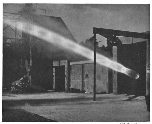
U.S. Navy photo This is what a test firing should look like. Note the mach diamonds in the exhaust stream.
