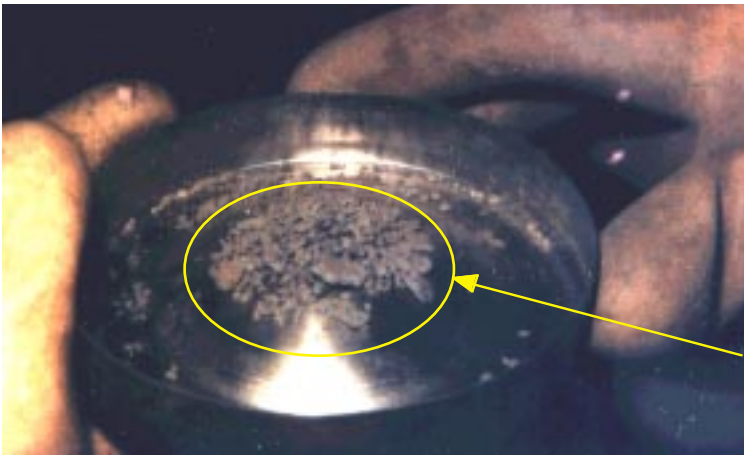
Fig. 7. Plutonium metal fines sieved from a crushed and blended MSE salt.
