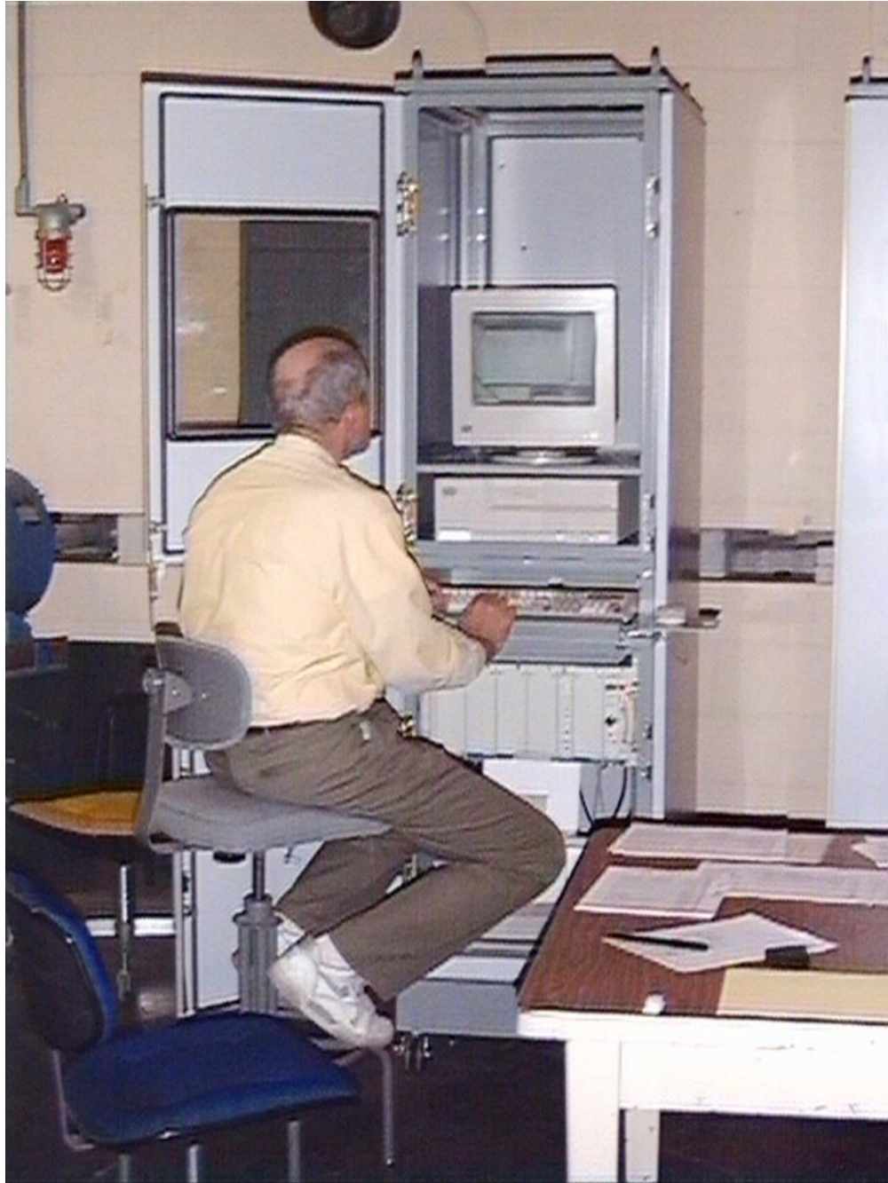
Fig. 3. Electronic cabinet for HENC showing the personal computer (PC) and the CI2150 multiplicity module.
