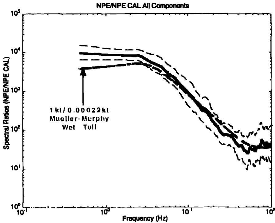
Figure 10: Comparison of the predict J spectral ratios from the Mueller-Murphy wet tuff model (thick/light dashed lines) and the NPE/NPE CAL empirical data (thick dark line) for model yields of 1 and 2 kt.
