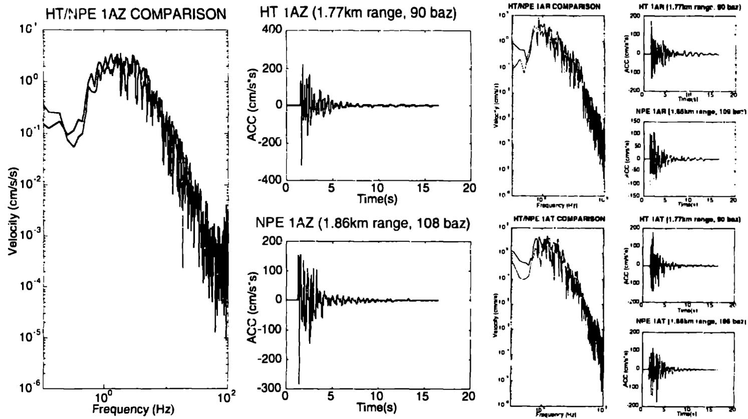
Figure 3: Comparison of the vertical accelerations from HT and NPE at Station IA (Figure 1) in the time and frequency domain (left). Radial (R) and transverse (T) comparisons made in the smaller format to the right.
