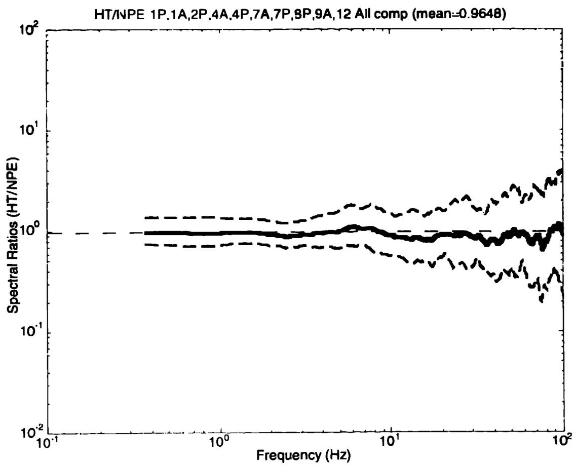
Figure 6: Mean spectral ratio (HT/NPE) determined averaging all station pairs (propagation path differences  $< 30\%$ ) and all components. Again the solid line is the mean with the plus or minus one standard deviation (log normal) characterizing the scatter in the individual estimates plotted as a dashed line.
