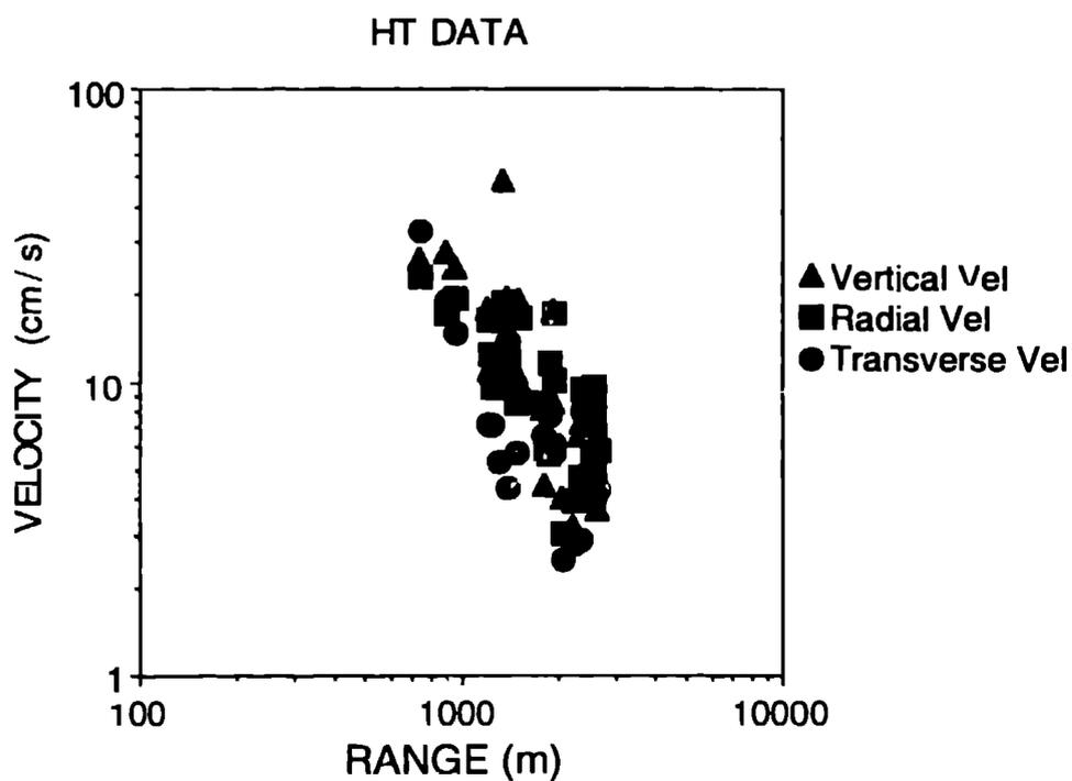
Figure 2: Peak velocity data for the radial (R), vertical (Z) and transverse (T) components of surface velocity observed at the stations diagrammed in Figure 1 from the explosions NPE CAL (top) and HT (bottom). Predictions plotted for the NPE CAL (open symbols) are from the models of Perret and Bass (1974).
