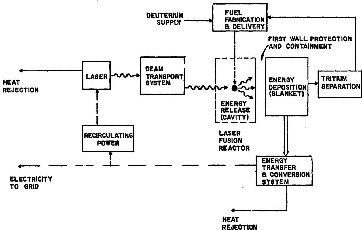
Fig. 3. Schematic energy and mass flow diagram.
