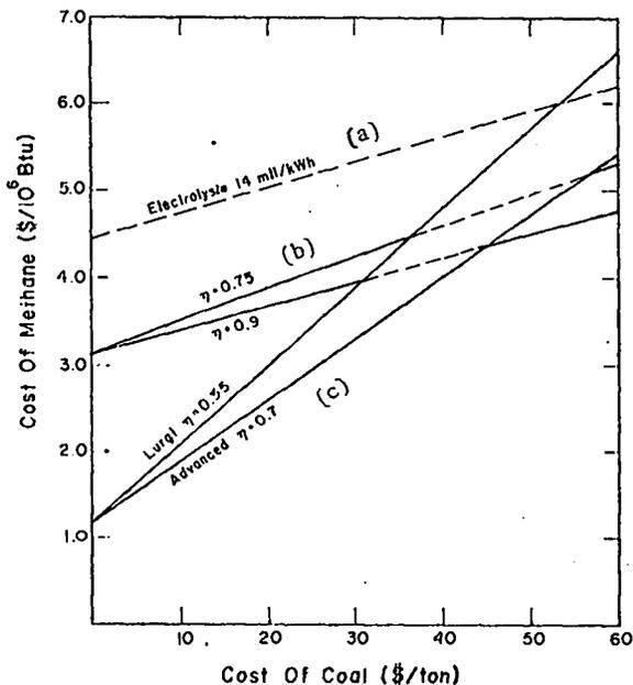
Fig. 11. Costs of producing methane by various methods as functions of the cost of feed coal: (a) electrolytically produced  $H_2$  followed by direct hydrogenation at  $\eta=0.9$ , (b) radiolytically produced  $H_2$  at  $\eta=0.35$  followed by direct hydrogenation with waste heat converted to electricity and sold for 14 mil/kWh, and (c) standard coal gasification ( $\eta$ =efficiency).
