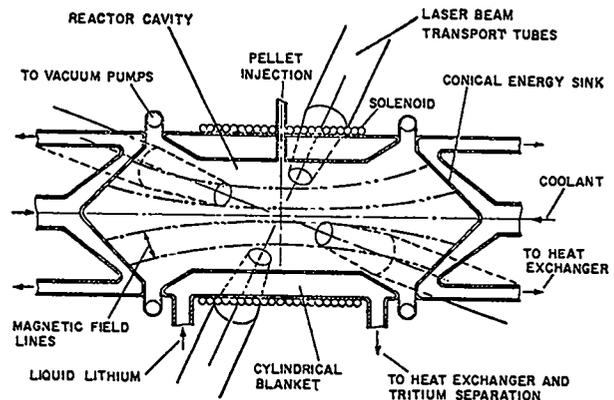
Fig. 2. Magnetically protected wall laser-fusion reactor concept.
