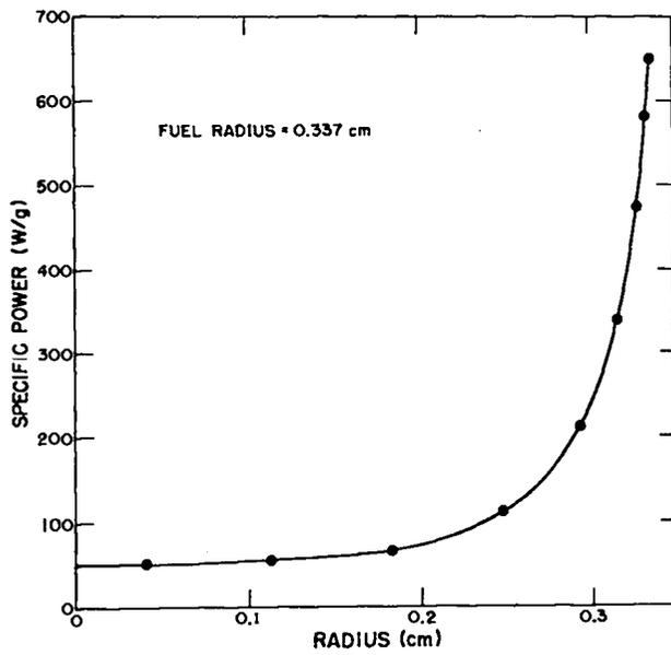
Fig. 467-2. Predicted radial power distribution in OWREX-14 fuel.
