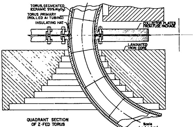
Fig. 4. Typical electrical feedpoint and primary of the torus.
