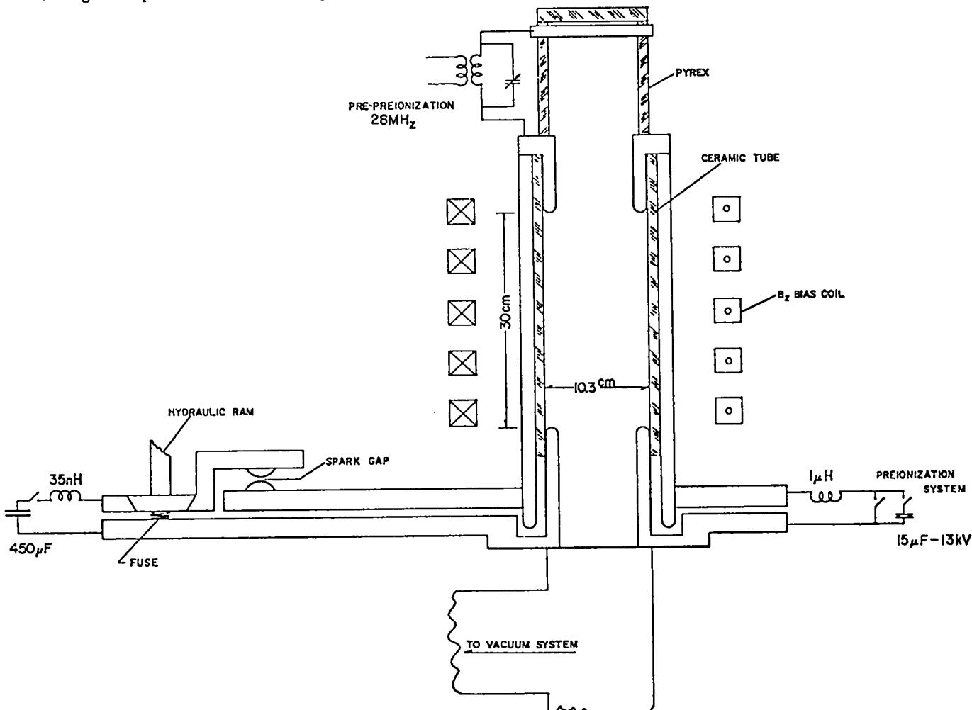
Fig. 1. Schematic diagram of the shock-heated linear  $z$ -pinch showing the technique of coupling a magnetic energy storage system to the  $z$ -pinch.
