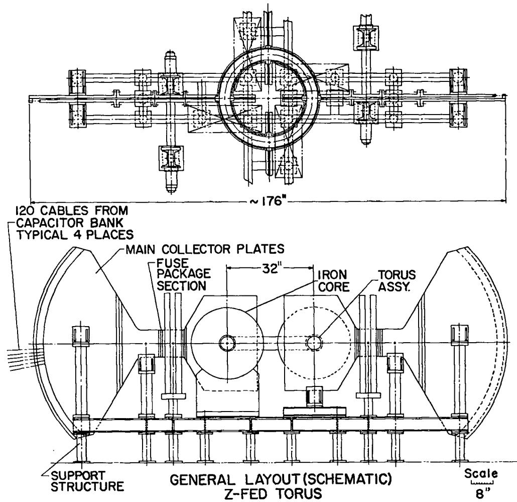
Fig. 6. Side elevation of the z-fed torus.
