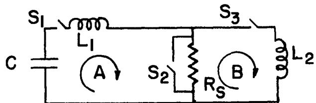
Fig. 2. Idealized circuit diagram of the magnetic energy storage system.
