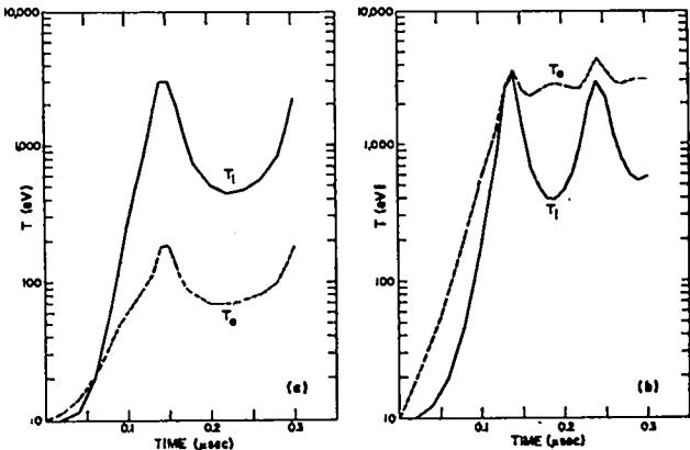
Fig. 3. Calculated ion and electron temperatures using (a) classical (b) anomalous resistivity.
