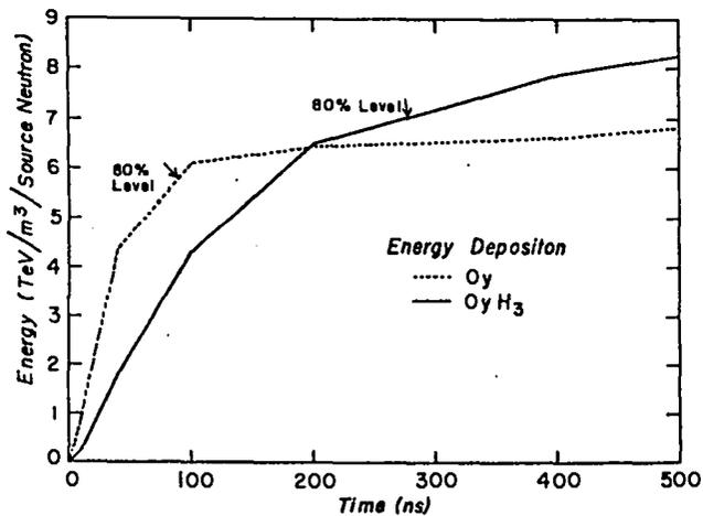
Fig. 2. Plot of the total energy deposited in the oralloy and  $OyH_3$  drivers as a function of time. The heating pulse is much slower in  $OyH_3$  and does not reach the 80% level until approximately 290 ns. These heating rates were calculated using the Monte Carlo code MCNG. The heating is in units of  $TeV/m^3$  per source' neutron.
