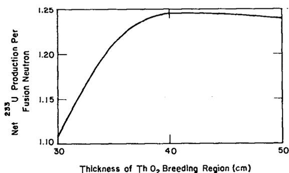
Fig.110. Net <sup>233</sup>U production per fusion neutron as a function of ThO<sub>2</sub> breeder-region thickness. Thorium contains 4 at.% <sup>233</sup>U.
