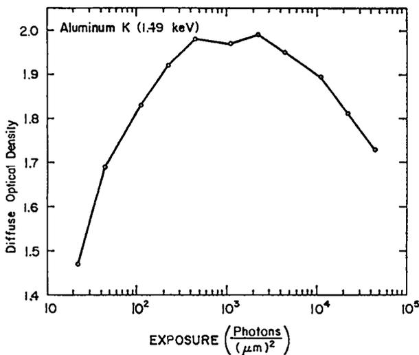
Fig. 97. Solarization of Kodak RAR 2490 film at 1.49 keV.
