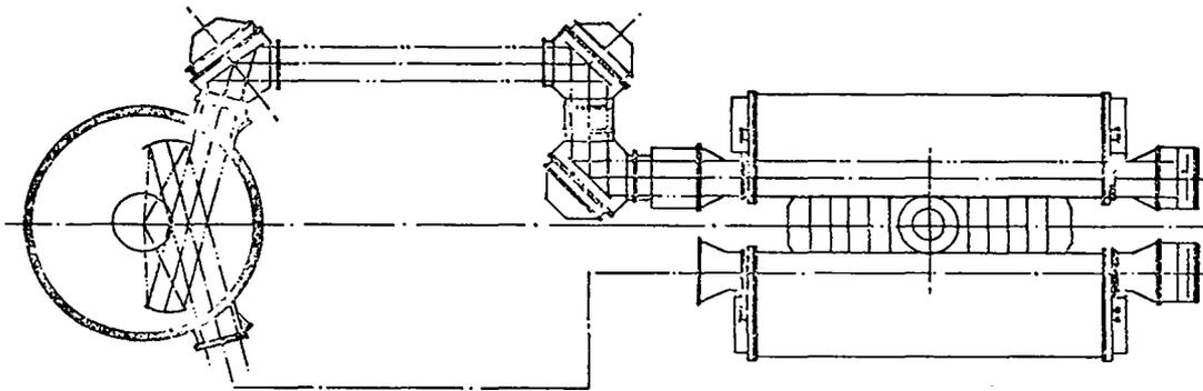
Fig. 73. Schematic of two-beam CO<sub>2</sub> laser and target chamber.
