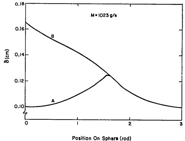
Fig.103. Lithium layer thickness for cases where mass supplied equals mass evaporated.
