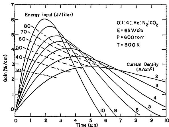
Fig. 10. Gain vs time for 0:1:4::He:N<sub>2</sub>:CO<sub>2</sub> mixture at 600 torr, 6 kV/cm. Gas temperature, 300 K.
