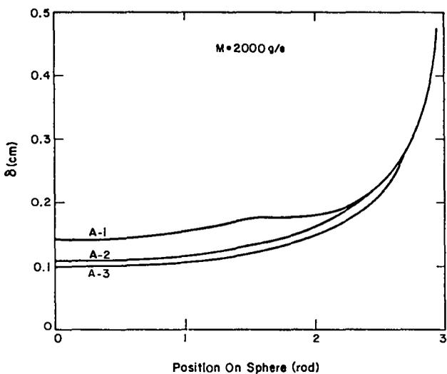
Fig.100. Lithium layer thicknesses corresponding to different step functions.
