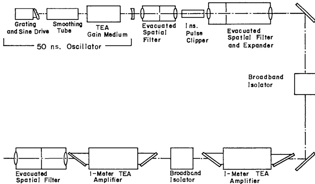
Fig. 29. Schematic layout of broadband Gigawatt Test Facility.
