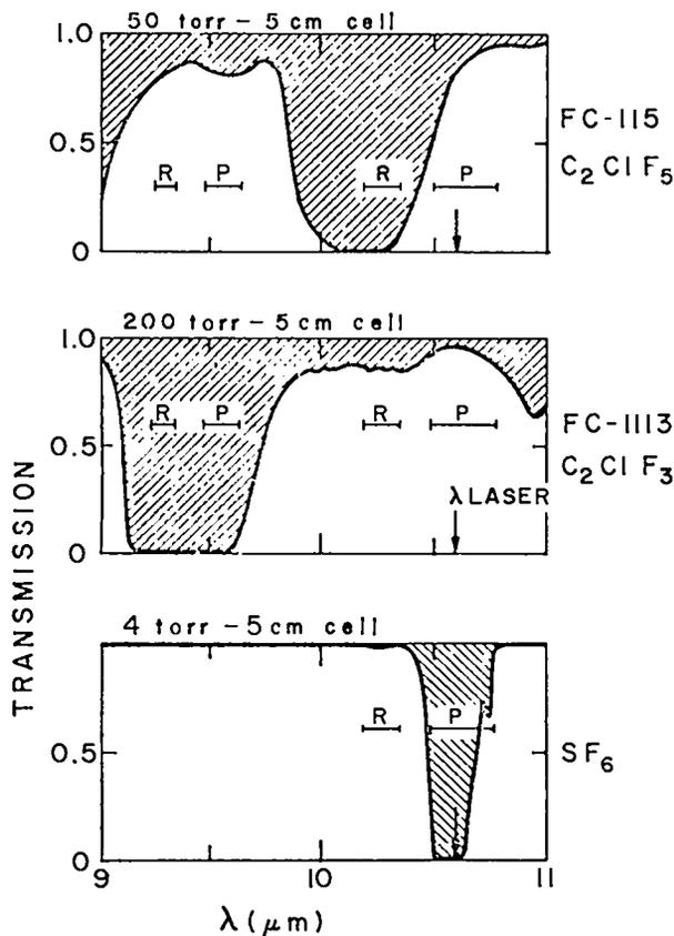
Fig. 2. Small-signal absorption spectra of  $\text{SF}_6$  and two fluorocarbons.
