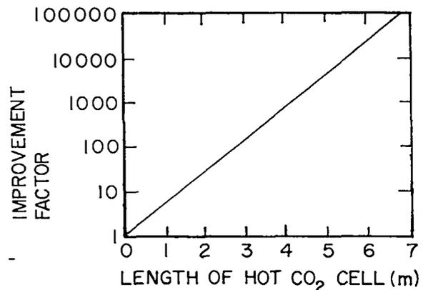
Fig. 39. Calculated improvement in contrast ratio of  $\text{CO}_2$  laser pulse through linear absorption in hot  $\text{CO}_2$  cell.
