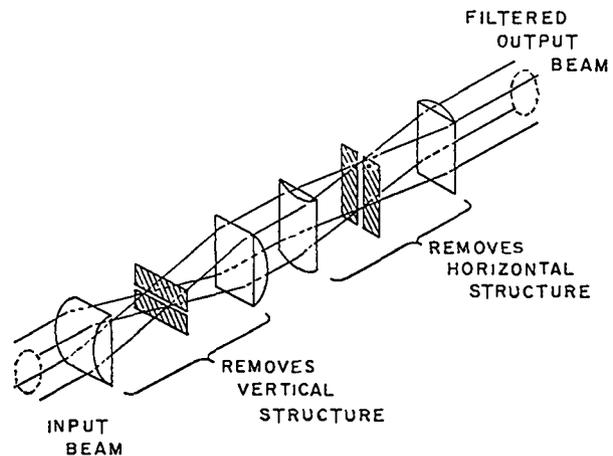
Fig. 33. Schematic of two-step cylindrical-optics spatial filter.
