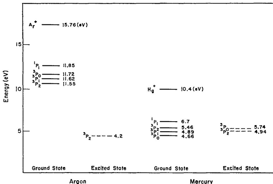
Fig. 53. Partial energy-level diagrams for argon and mercury.
