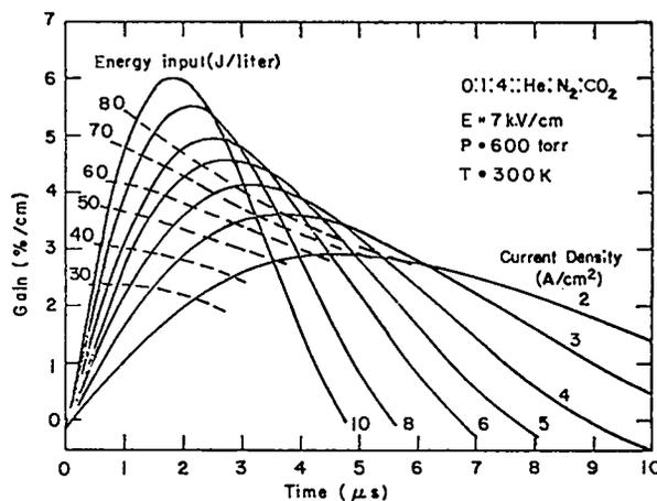
Fig. 11. Gain vs time for 0:1:4::He:N<sub>2</sub>:CO<sub>2</sub> mixture at 600 torr, 7 kV/cm. Gas temperature, 300 K.
