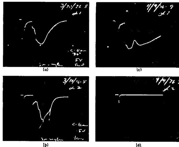
Fig. 68. Time histories of low emission for single and double foils; (a) and (b) show front and back ion emission, respectively, for a single 3- $\mu\text{m}$ -thick foil; whereas, (c) and (d) show front and back ion emissions, respectively, for a 0.1- to 3- $\mu\text{m}$ -thick double foil separated by 75  $\mu\text{m}$ .
