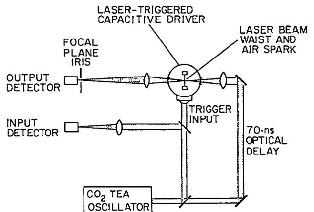
Fig. 36. Setup for studying electrically driven plasmas.
