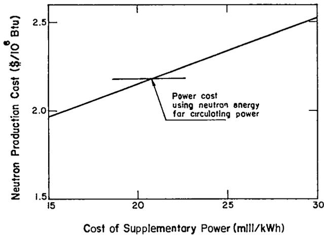
Fig. 111. Neutron production cost (1973 dollars) as a function of the cost of supplementary electrical power purchased.
