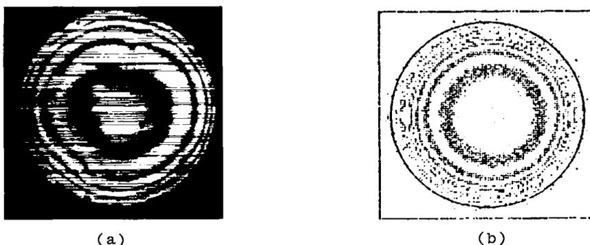
Fig. 78. Interferograms of a nonconcentric thick-walled microballoon. (a) Photomicrograph from a Jamin-Lebedev interferometer; measured wall thickness,  $3.1 \mu\text{m}$ ; measured diameter,  $99 \mu\text{m}$ ; measured nonconcentricity,  $0.16 \mu\text{m}$  (i.e.,  $0.32\text{-}\mu\text{m}$  wall-thickness variation). (b) Computer-generated interferogram calculated from measured parameters.
