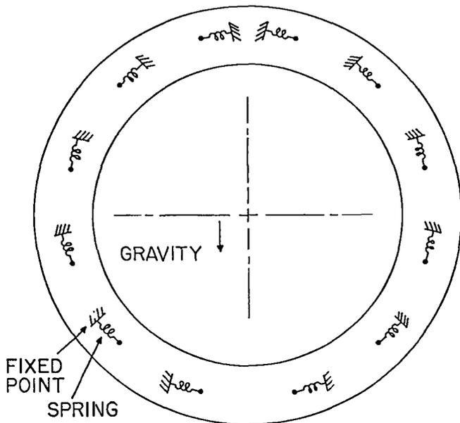
Fig. 15. Schematic of tangential spring support for mirrors.
