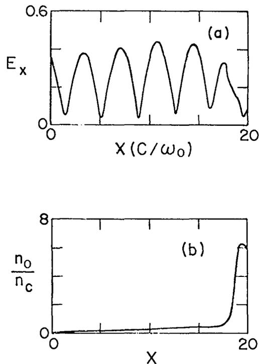
Fig. 76. Results of laser-plasma interaction simulation. Simulation parameters are the same as in Fig. 75, except that the incident laser is polarized in the x-y plane (plane of incidence) at 23° to normal; (a) amplitude of the x-directed electric field at  $t = 200 \omega_0^{-1}$  as a function of position; (b) self-consistent density profile.
