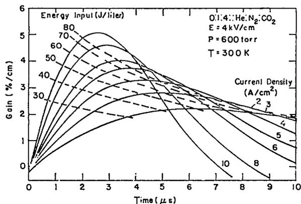
Fig. 8. Gain vs time for 0:1:4::He:N<sub>2</sub>:CO<sub>2</sub> mixture at 600 torr, 4 kV/cm. Gas temperature, 300 K.
