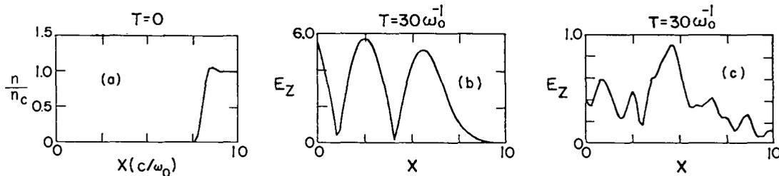
Fig. 74. Two-dimensional particle-in-cell simulation; (a) Initial density profile; (b) incident laser electric-field amplitude at  $T = 30\omega_0^{-1}$ , and (c) the most unstable  $k_y = 3\omega_0/c$  scattered wave.
