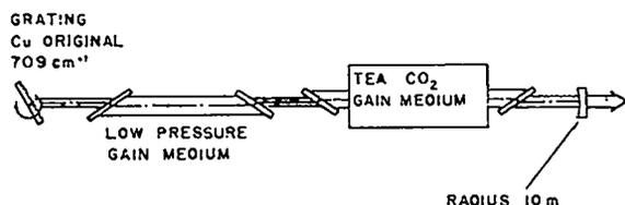
Fig. 22. Single-line cw smoothing-tube stabilized  $\text{CO}_2$  oscillator.
