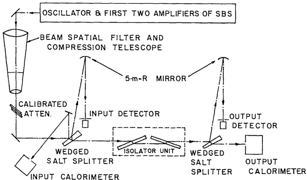
Fig. 35. Experimental setup for characterization of Isolator properties.
