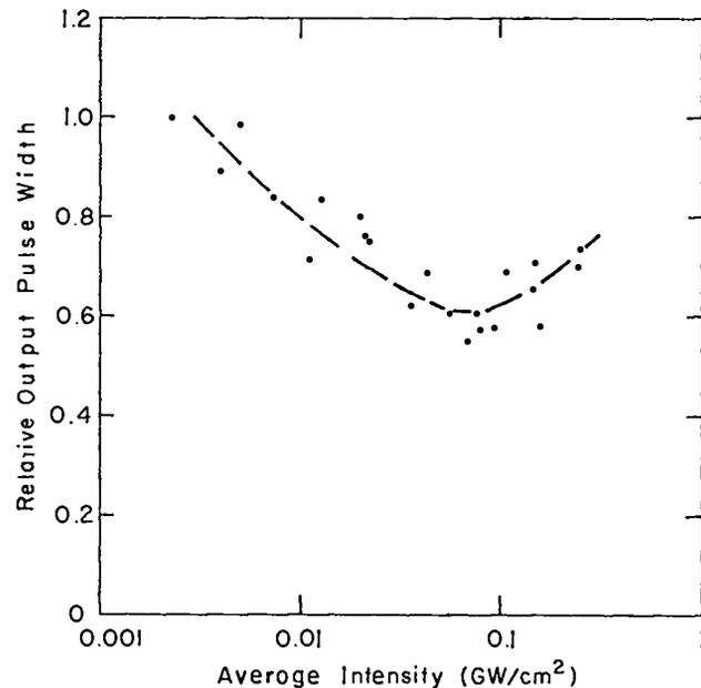
Fig. 28. Pulse shortening measured in p-type germanium. The horizontal axis is intensity in the air just prior to the Brewster-angle sample.
