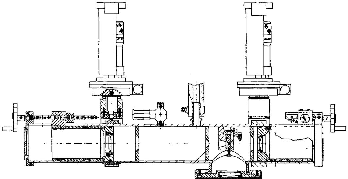
Fig. 31. EG&G mechanical design for a typical spatial-filter telescope.
