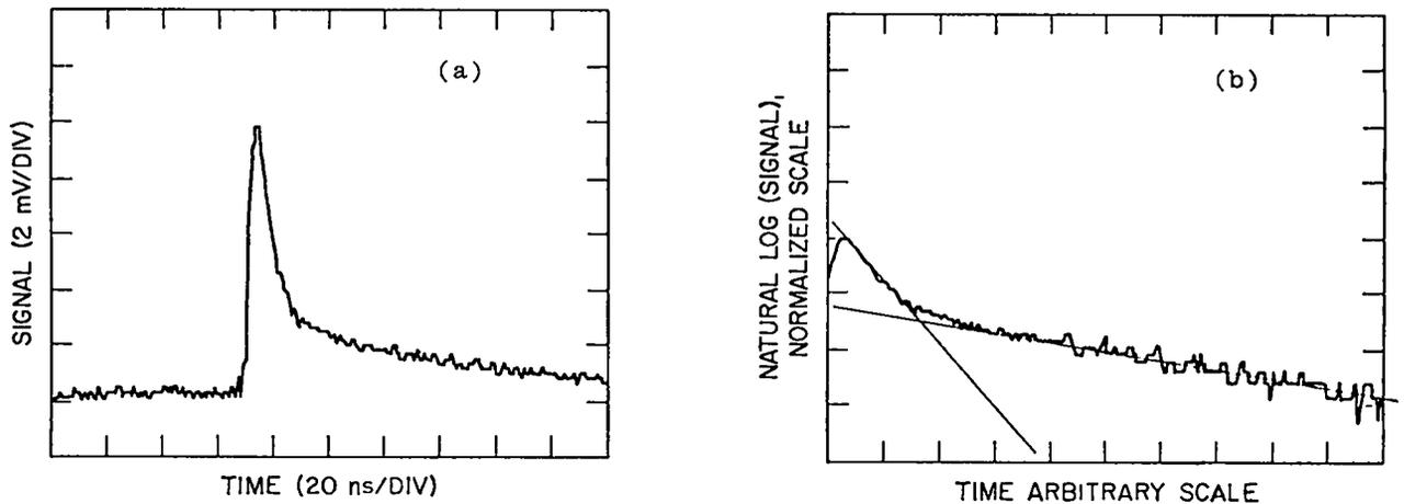
Fig. 48. Photodiode signal for 200-psia xenon using a 1500-psia Ar:150-psia Kr:1200-torr H<sub>2</sub> mix to fill the optical source chamber to 1000 psia; (a) linear scale; (b) logarithmic scale.
