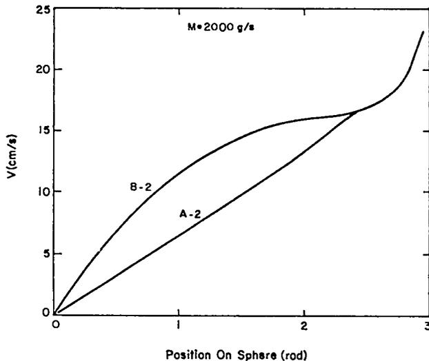
Fig.102. Lithium tangential flow velocity for step and linear mass flow-rate functions,  $m_s(\theta)$ .
