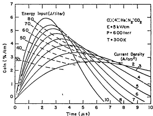
Fig. 9. Gain vs time for 0:1:4::He:N<sub>2</sub>:CO<sub>2</sub> mixture at 600 torr, 5 kV/cm. Gas temperature, 300 K.
