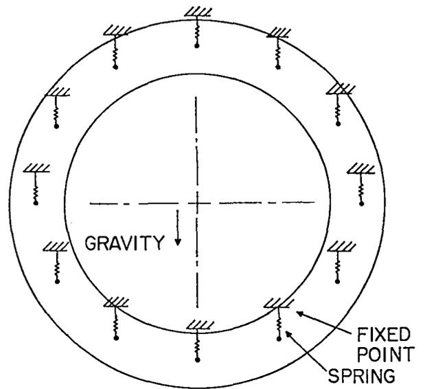
Fig. 16. Schematic of vertical spring support for mirrors.
