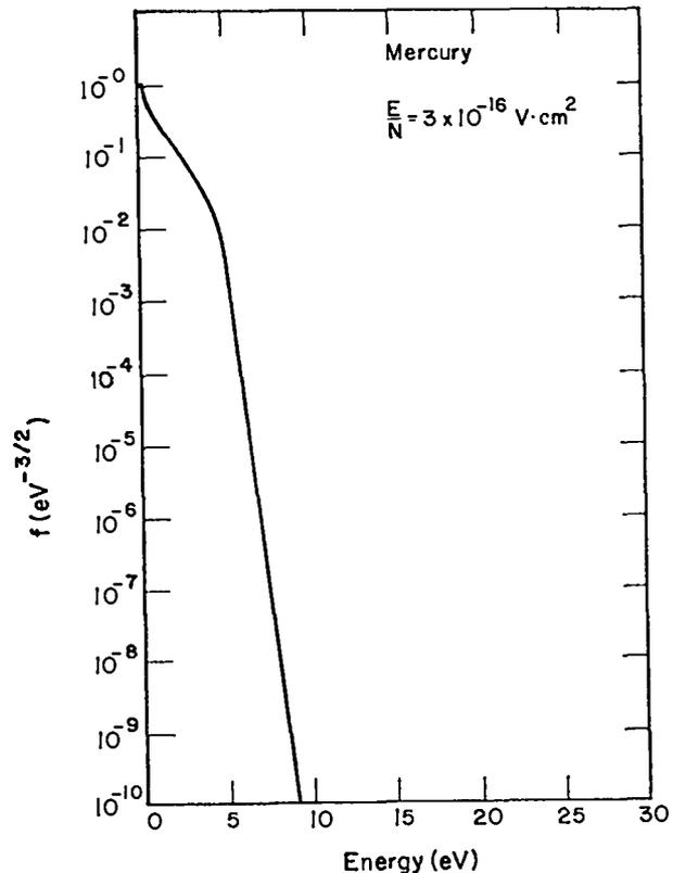
Fig. 56. Electron energy-distribution function in mercury for  $E/N = 3 \times 10^{-16} \text{ V}\cdot\text{cm}^2$ .
