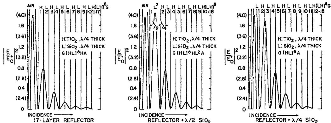
Fig. 63. Standing-wave electric-field intensities in three  $\text{TiO}_2/\text{SiO}_2$  multilayer reflectors: (a) 17 layers; (b) same as (a) plus  $\lambda/2$ -thick  $\text{SiO}_2$  overcoat; and (c) same as (a) plus  $\lambda/4$ -thick  $\text{SiO}_2$  overcoat.
