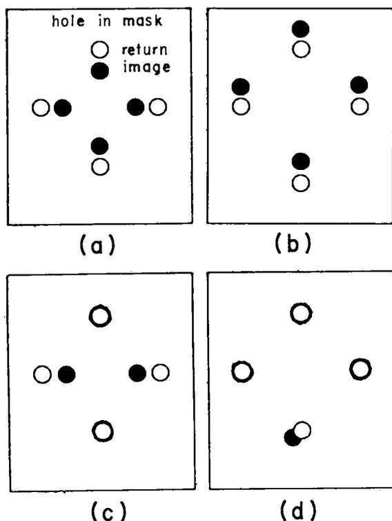
Fig. 3. Typical displays from Hartmann Mask beam-alignment system. (a) Beam focus in front of sphere center; (b) beam focus above sphere center; (c) paraboloid axis not parallel to incoming beam in horizontal plane; (d) wavefront error in beam or paraboloid.
