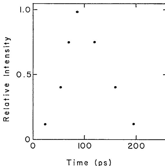
Fig. 26. An ultrashort FID pulse. This is the streak-camera record corrected for the nonlinearity of the CS<sub>2</sub> Kerr-cell upconverter. Camera response characteristics are still present.
