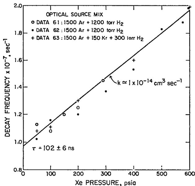
Fig. 49. Decay frequency of  $I_U:O_U^-$  vs xenon pressure.
