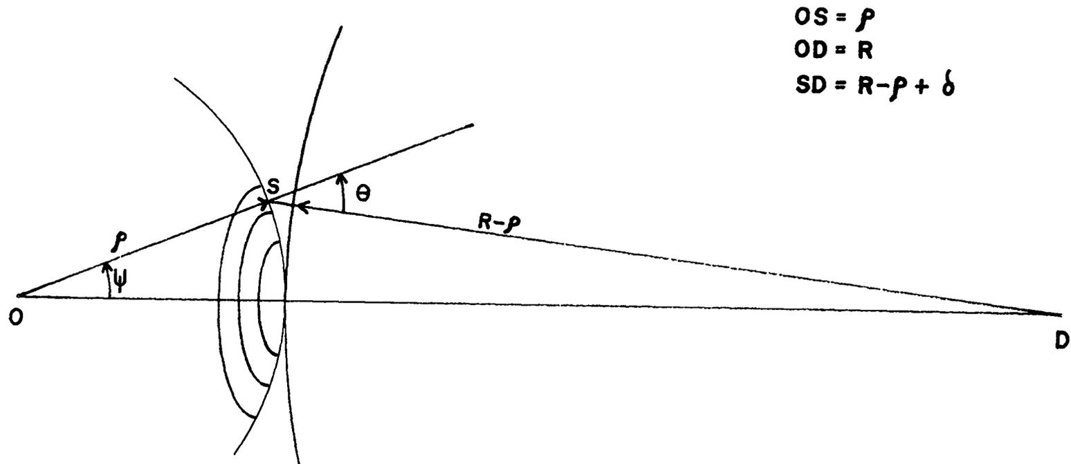
Figure 3. Path difference of signals from a spherical source.
