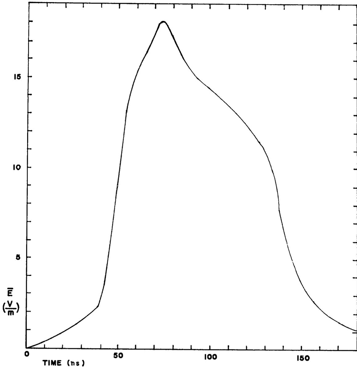
Figure 1. Fast electromagnetic pulse form.
