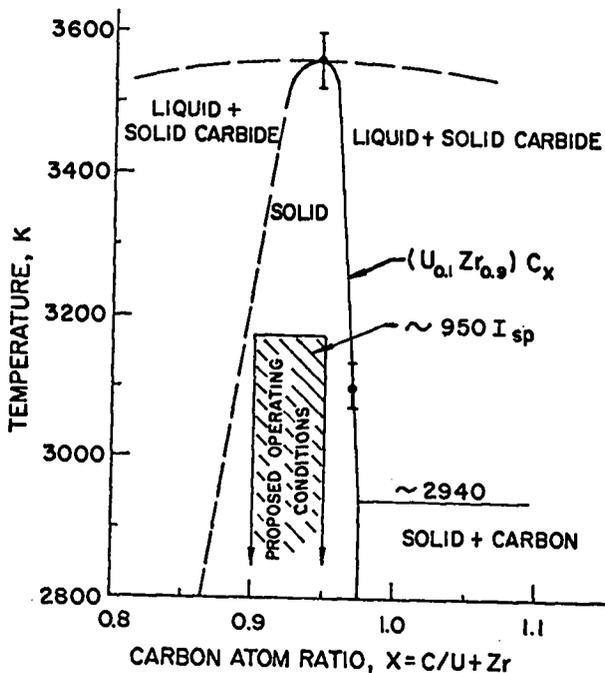
Fig. 16. Pseudobinary phase diagram for  $(U_{0.1}Zr_{0.9})C_x$ .
