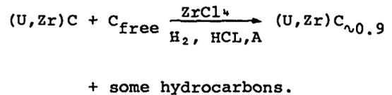
A third method, a combination of the first two, was the most practical. The free carbon was removed by flowing hydrogen at a temperature of 2200 to 2300 K for 40 to 60 h. The elements were then impregnated with zirconium in a gas mixture of the following composition (vol%): ZrCl<sub>4</sub>, 1.8%; H<sub>2</sub>, 8.2%; CH<sub>4</sub>, 0.02%; HCl, 0.10%; and Ar, 89.9%. The temperature of impregnation was ~ 1900 K.
