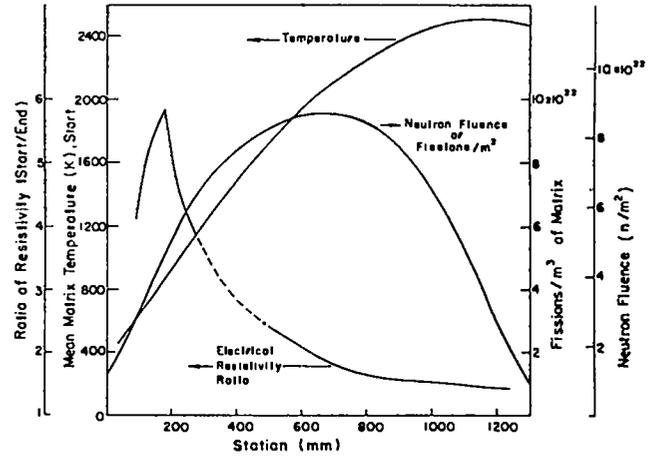
Fig. 11. Fuel-element environment vs length: temperature, fissions, and fast-neutron fluence ( $>0.18$  MeV). Also plotted is the change in room-temperature electrical-resistivity ratio for a composite fuel element, start to end, of the NF-1 reactor run.
