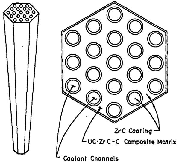
Fig. 1. Full-length and cross-section views of composite fuel element. Length, 1.32 m; across-flats, 19 mm; coolant-channel diameter, 2.3 mm; mass,  $\sim 1.1$  kg; and volume,  $284 \times 10^{-6}$  m<sup>3</sup>.
