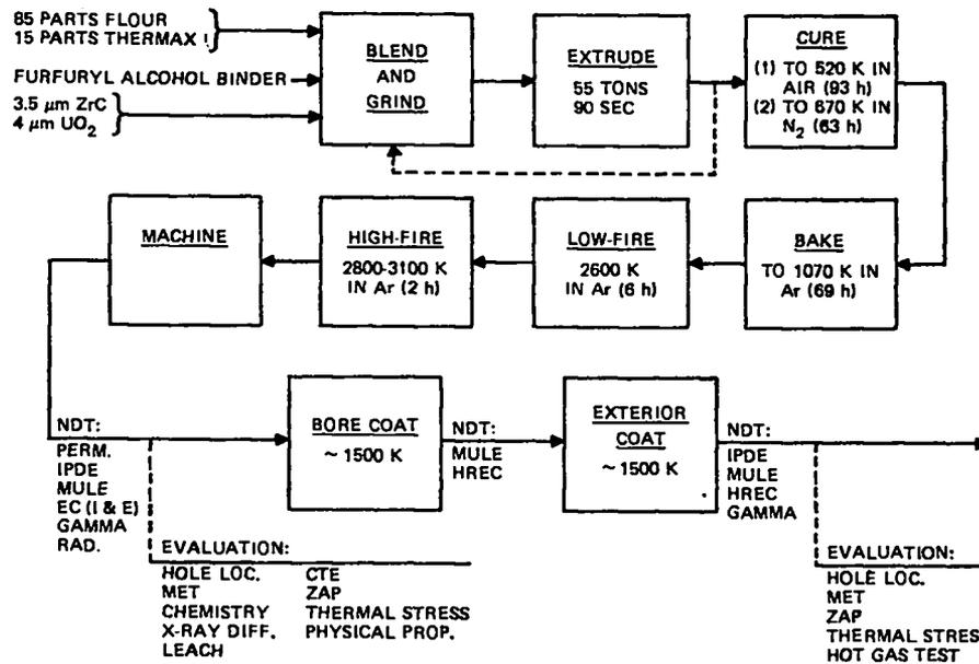
Fig. B3. Preparation and evaluation of composite fuel elements.
