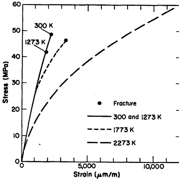
Fig. C1. Stress-strain data from room temperature to 2273 K for a (U,Zr)C-graphite composite of 30-vol% carbide content and 630 kg/m<sup>3</sup> uranium loading.
