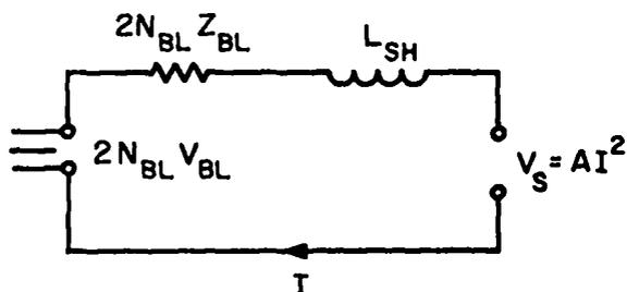
Fig. 6. Circuit diagram of the shock-heating circuit.
