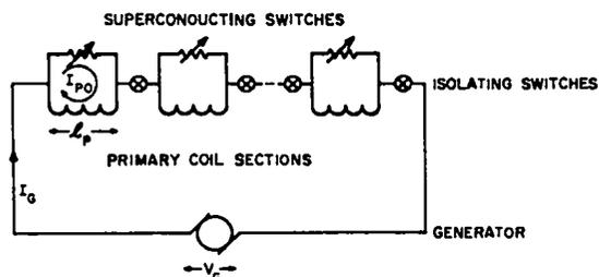
Fig. 11. Charging circuit for superconducting primary coils.
