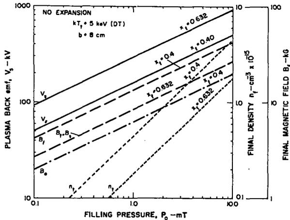
Fig. 2. Plasma heating parameters versus filling pressure for various compression ratios  $x_f$ .
