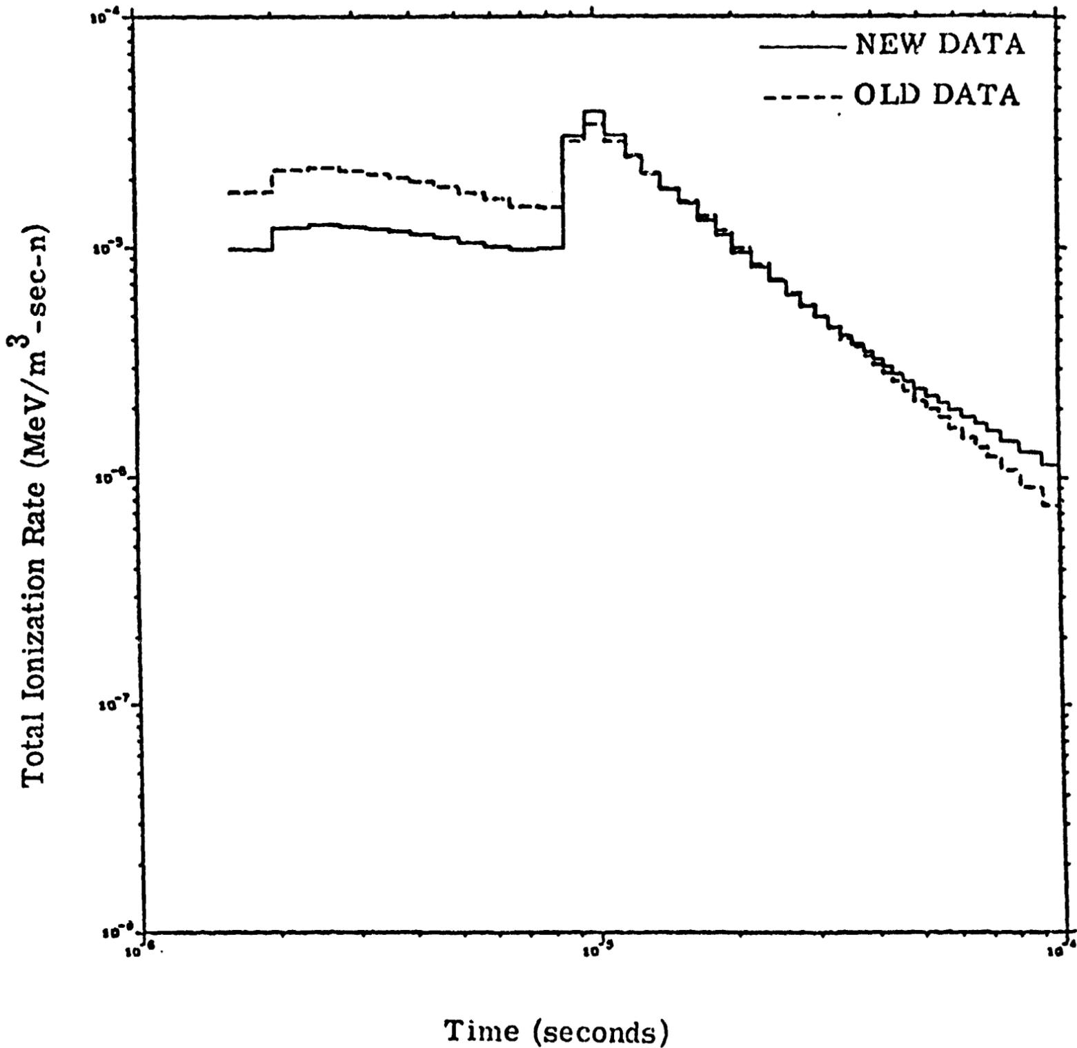
Fig. 8. Calculation by Sargis et al.<sup>22</sup> of the total neutron and gamma-ray ionization rate at 480m from a thermonuclear source. The calculations were performed using an older ENDF/B evaluation of the neutron cross sections combined with gamma-ray production data from the United Nuclear Corp.<sup>23</sup> and with the more recent ENDF/B(3) evaluations of Young and Foster.<sup>2,24</sup>
