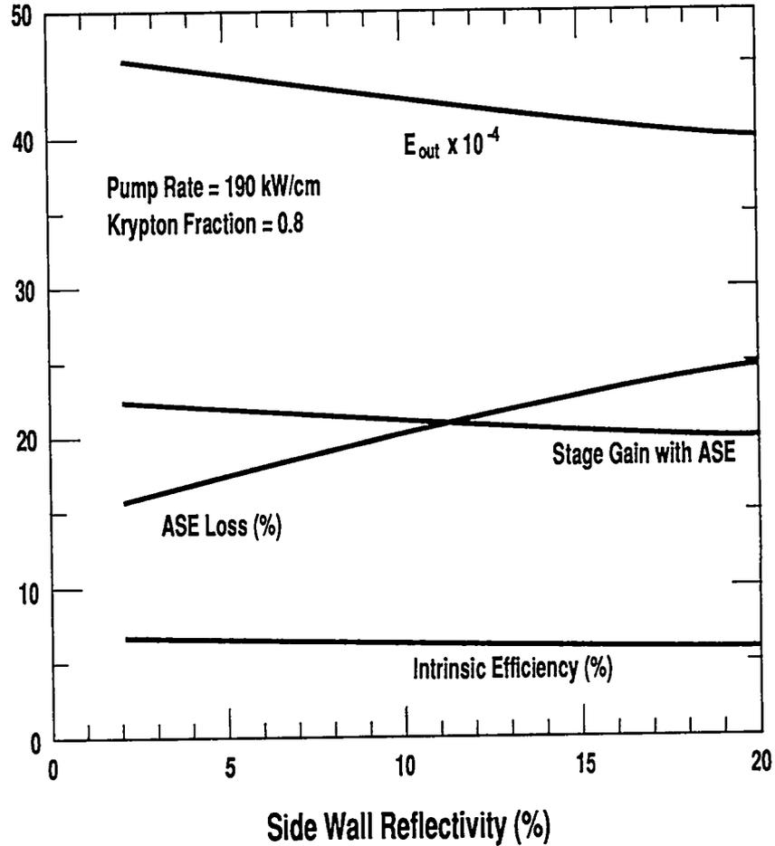
Figure 10 shows a plot of performance of the large amplifier as a function of side-wall reflectivity for a pump rate of 190 kW/cm<sup>3</sup> and a krypton fraction of 0.8. The effect of reducing the side-wall reflectivity is to reduce the losses due to ASE. Figure 10 shows that our desired performance of 410 kJ can be achieved at a side-wall reflectivity of 20%, but that significantly higher energy output could be achieved if the wall reflectivity could be reduced to 5%.
