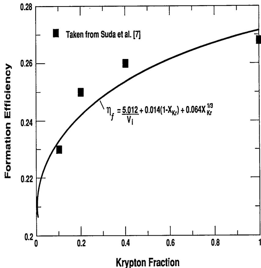
Following Shaw<sup>2</sup>, if one assumes ionization is the sole route to excitation and that the chemistry is 100% efficient, the formation efficiency can be approximated by
