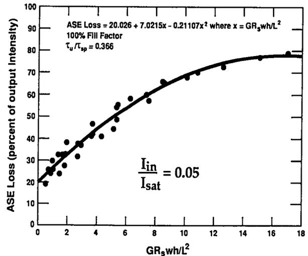
Fig. 7. Shown is a global approximation to the amplified spontaneous emission loss in large KrF amplifiers. The approximation will give answers that are normally within  $\pm 20\%$  of Leland's<sup>10</sup> three-dimensional extraction.
