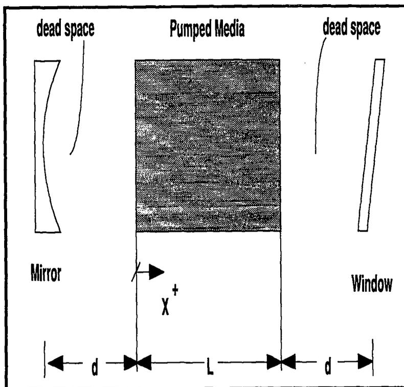
itself to pass through the laser media a second time before it exits through the window. The laser media is bounded on each end by unpumped zones that are used to protect the mirror and window from pumping electrons and from the atomic fluorine in the pumped volume. Rice et al.<sup>1</sup> have shown that the differential equations governing the growth of the intensity of an extracting beam as a function of the spatial coordinate is given by
