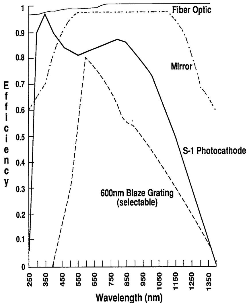
the fiber optic cable, which at 850-nm wavelength and a cable length of 10 m is 300 ps, as verified experimentally. Spectral resolution is limited by the streak camera; for the various gratings this becomes, 3.64 nm, 1.21 nm, and 0.61 nm for the 100 g/mm, and 600 g/mm, respectively. ■
