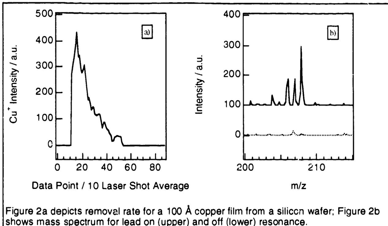
Figure 2a depicts removal rate for a 100 Å copper film from a silicon wafer; Figure 2b shows mass spectrum for lead on (upper) and off (lower) resonance.
