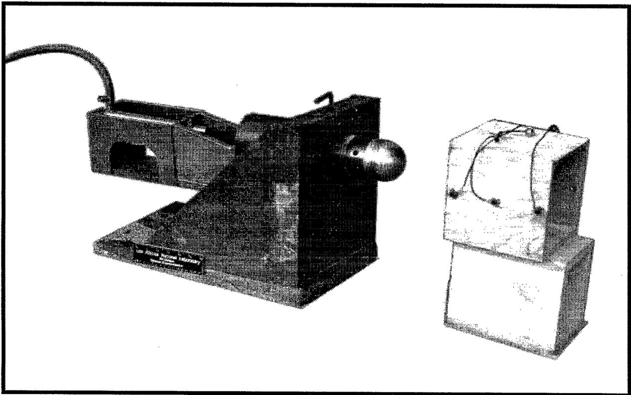
Figure 3: Spigot gun and photodiode velocity screen box.
