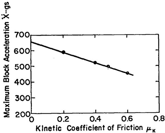
Fig. 12. Effect of kinetic coefficient of friction.
