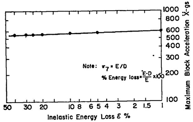
Fig. 13. Effect of inelastic energy loss.
