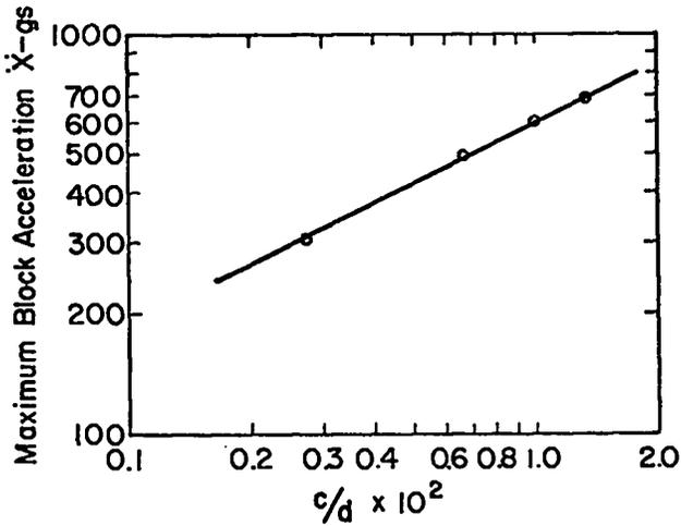
Fig. 11. Effect of block clearance gap.
