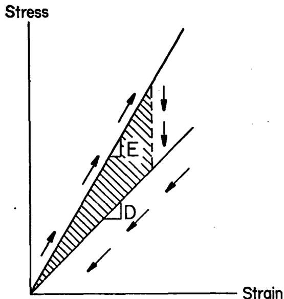
Fig. 4. Inelastic energy loss model.
