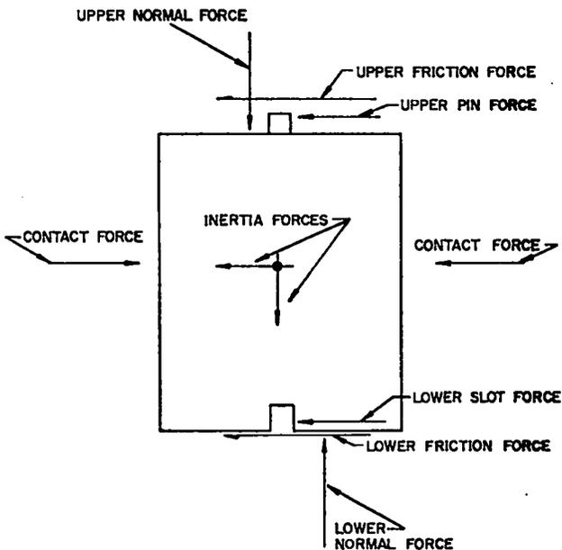
Fig. 1. Forces acting on core block.
