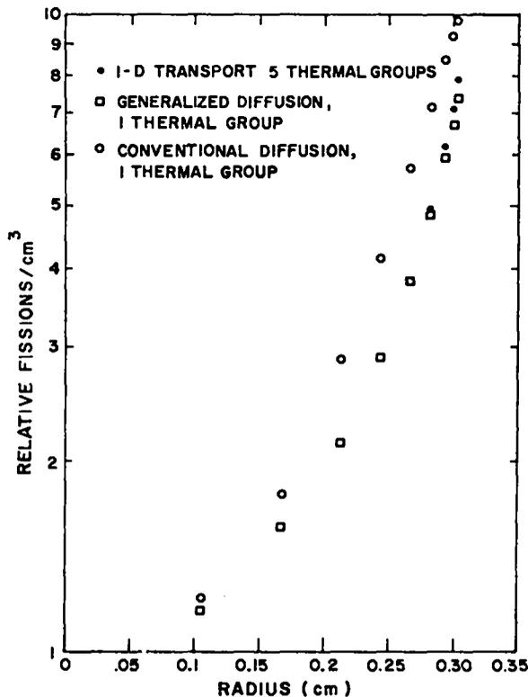
Fig. 10. Radial fission density through experimental pin of Example 4.
