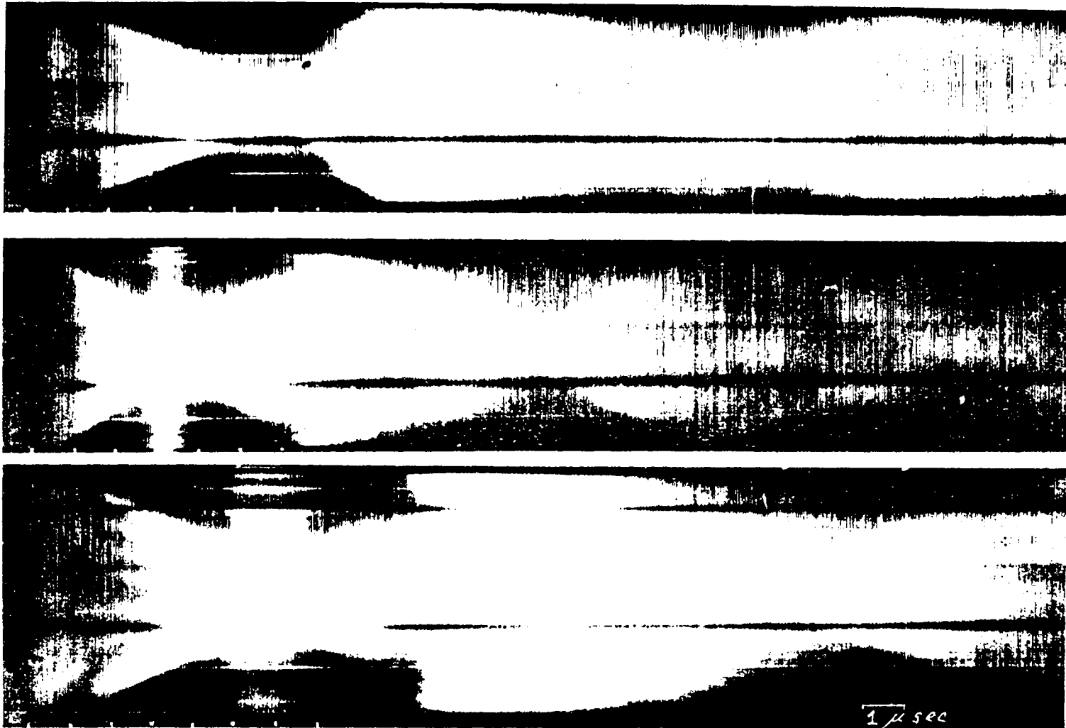
Shocks (a) pinches (b) and combination shocks and pinching (c) observed in (a and b) a 3" diameter 17" long discharge tube with a 5" diameter 8 wire coaxial return, ((c) is with a 4.5" tube in the 5" diameter coaxial return) 10 - \mu f condensers each coaxially connected to a spark gap switch. (a) D_2 at 1200 \mu Autovac pressure 3 KV (b) D_2 at 600 \mu Autovac pressure 8 KV (c) D_2 at 400 \mu Autovac pressure 14 KV - 4.5" tube
