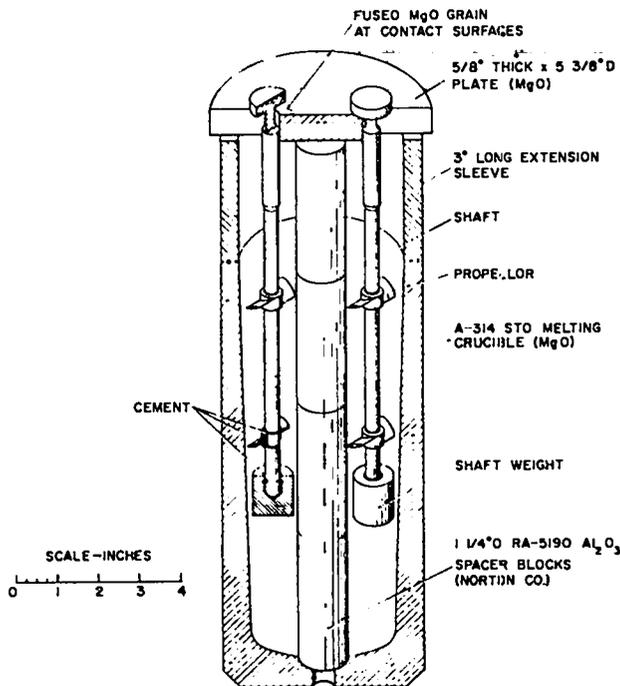
Fig. 4. Setup for firing stirrer assemblies.
