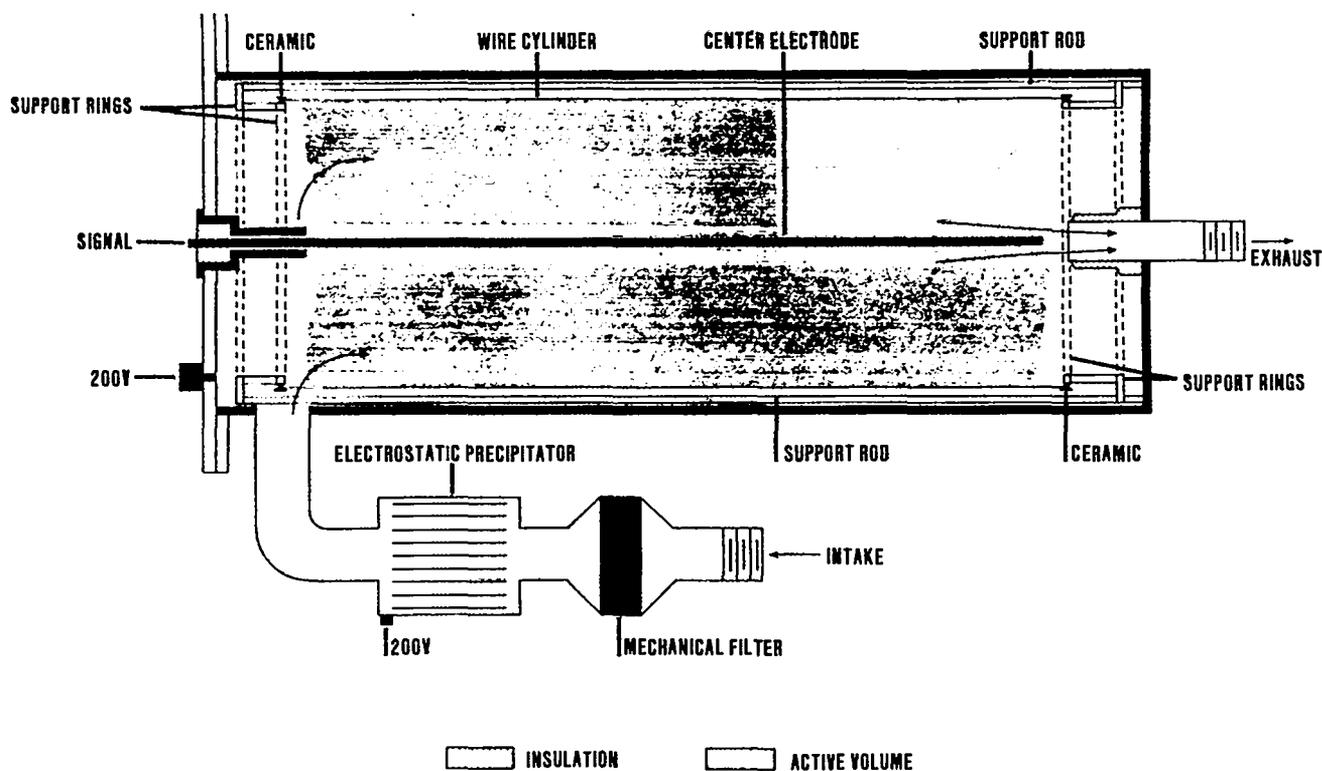
Fig. 5. Detailed drawing of the improved Kanne chamber.
