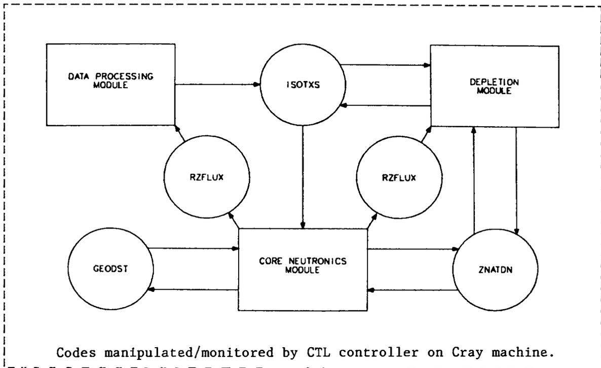
Fig. 30. DANDE code system for reactor core analysis.
