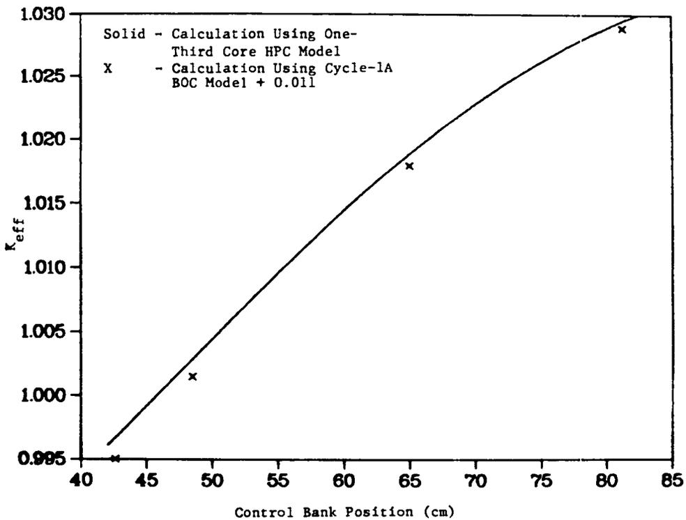
Fig. 31. FFTF control bank worth (no depletion).
