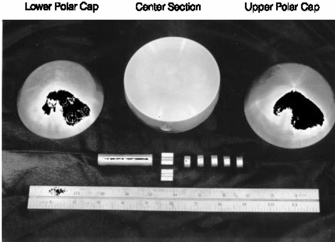
The experimental setup is shown in Figure 2. Assembly was accomplished by raising the lower polar cap and lower safety block up into the assembly. Rapid disassembly, in the event of a scram, was accomplished by retracting the upper and lower safety block as well as the control rod (Reference 1). Reactivity was adjusted using the glory hole filler pieces.
