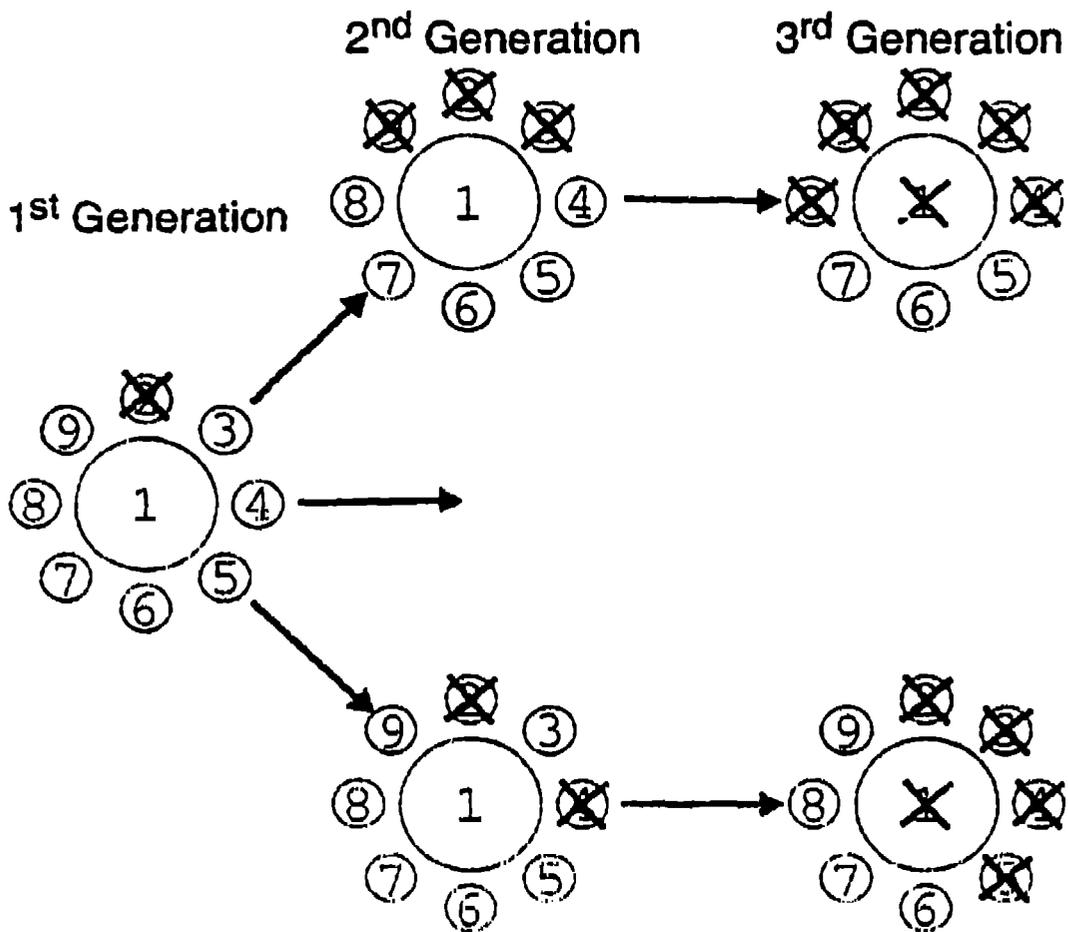
Figure 2 - Basic accident model showing possible propagation scenarios.
