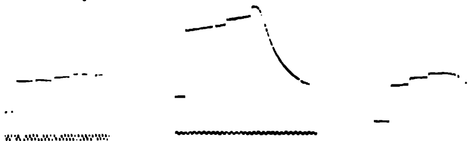
Fig. 22. Records showing shock wave arrivals in fused quartz.
