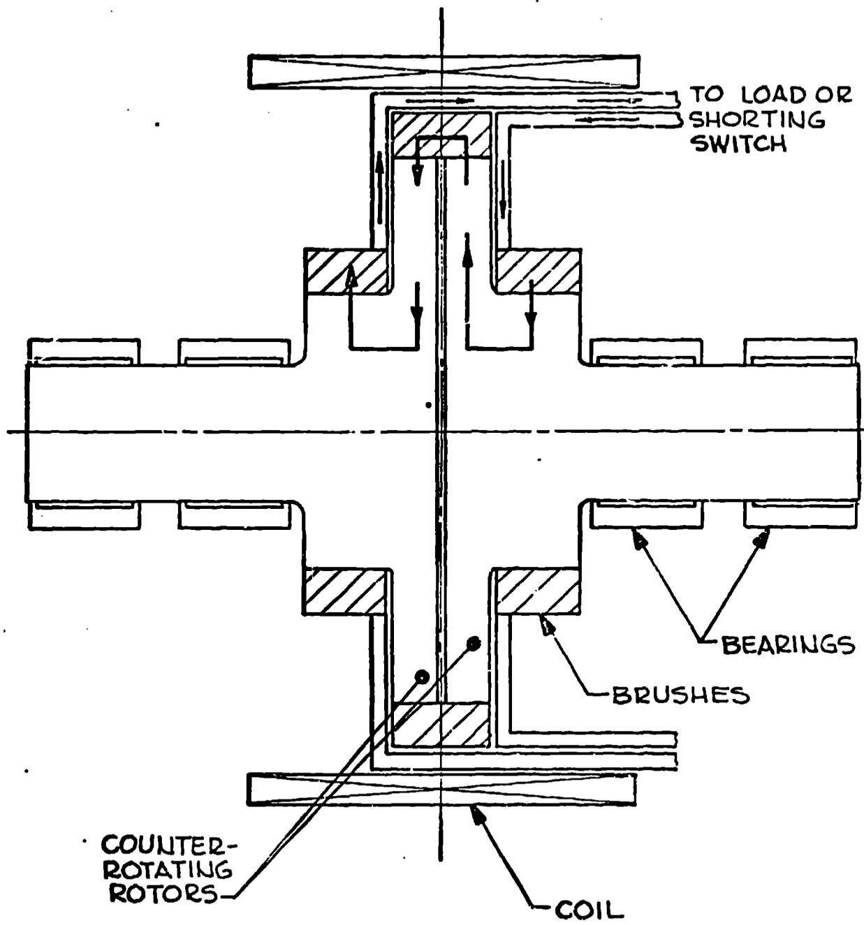
Fig. 3 Fast Discharging Homopolar Machine
