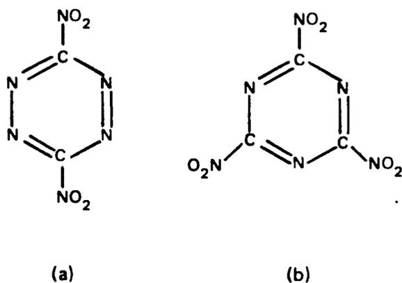
Fig. 2. Nitroheterocycles (a) 3,6-dinitro-*s*-tetrazine and (b) 2,4,6-trinitro-*s*-triazine.
