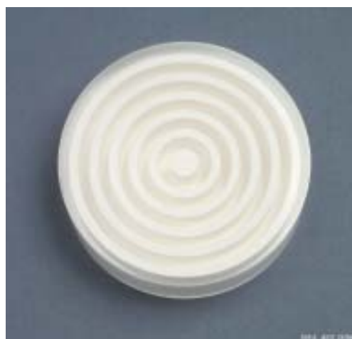
Figure 2. Eljen EJ410-P fast scintillator.
